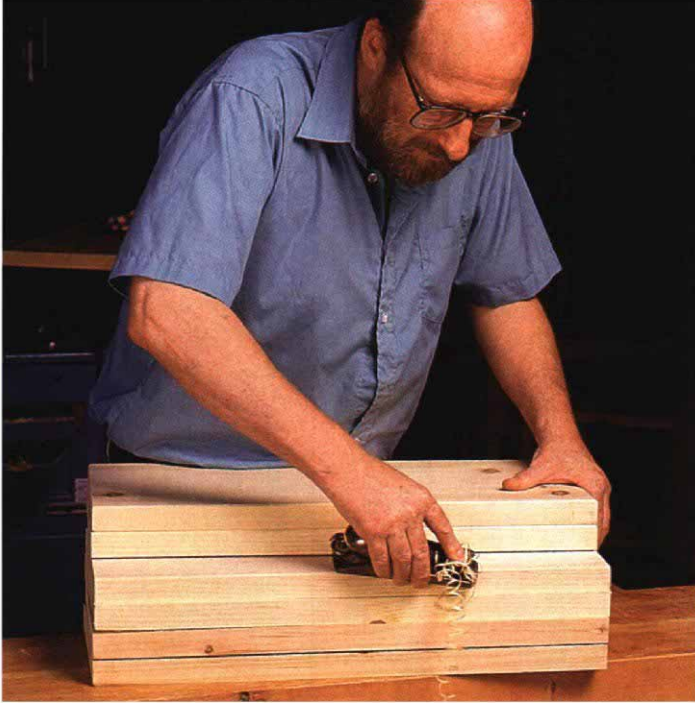
The block plane makes short work of chamfering edges. Chamfer the top board in the stack, offset it a few inches to get at the next board, and carry on down the whole stack before turning or rotating to a new corner.
