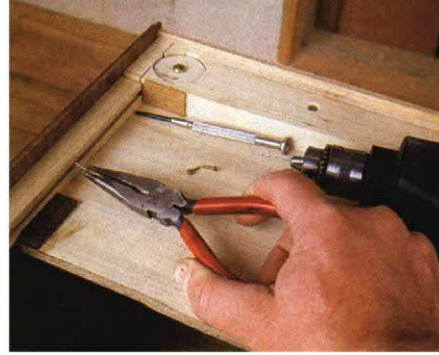
To allow for wood movement in the side of his case, Greef fastens a guide channel by first drilling oversized holes in the guide. Then he installs three screws within the channel using needle-nose pliers and a tiny screwdriver. To complete the door-guide system, he glues a pair of walnut skids at the front of the case and a pair of cork bumpers at the rear.
