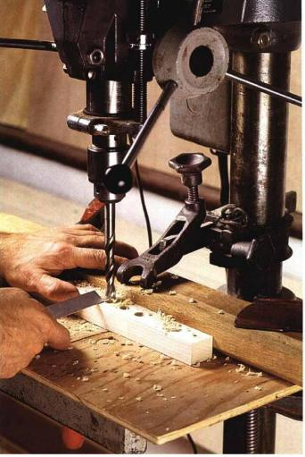
**Using a metal rule,** Maas double checks each hole's edge distance for the series he bored with a machine-spur bit chucked in his drill press. A fence, clamped to the table with a hold-down, keeps the workpiece aligned while the machine's depth gauge (next to the feed lever) ensures that the holes are uniformly deep.
