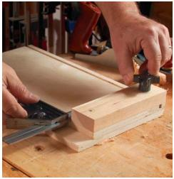
**Squaring up is easy.** To set up for shooting, loosen the adjustment knob and square the fence to the edge of the jig with a combination square. The first few passes with the plane will flush the fence to the edge of the jig, creating a zero-clearance back stop for planing parts.
