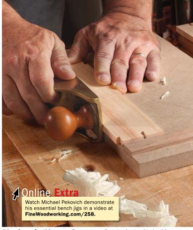
A low fence for thin parts. Because small parts also tend to be thin, the fence only protrudes  $\frac{3}{16}$  in. above the deck (left). It can be difficult to maintain a square edge while planing thin stock, so Pekovich lays the part and plane on their sides to make edge-planing easier (above).
