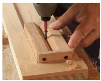
**V-blocks support stock at an angle.** For shaping or chamfering long, narrow parts, screw a pair of beveled blocks to each end of the jig (above). The front block has an end stop screwed to the face to hold the stock in place while shaping (right).
