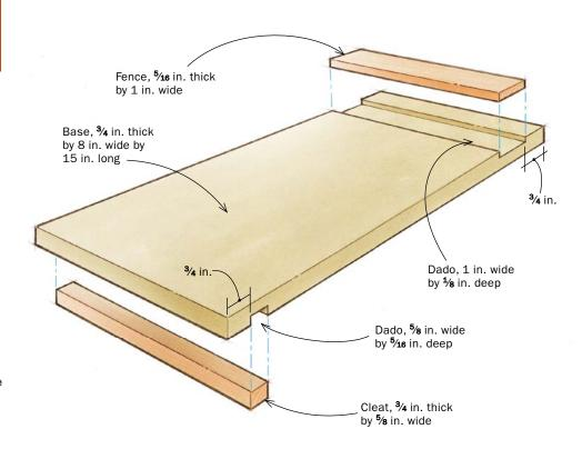
Dadoes simplify assembly. The fence and cleat on this jig, as well as those on the saw hook (opposite page), are glued into shallow dadoes in the bases. This ensures a sturdy, square glue-up of the jig parts.
