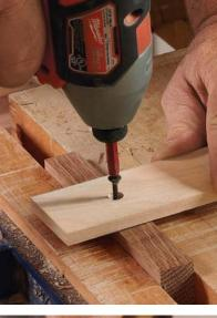
Two scraps and a screw are all you need. The T-square jig consists of a long fence attached to a cleat with a recessed screw. To use it, clamp the cleat in your vise and secure the opposite end with a clamp or benchdog (below).
