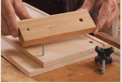
**Drilling for the fence.** Because the oversize hole only allows for slight adjustment, the fence holes in the base should be drilled as accurately as possible. To make this easier, pre-drill the fence, clamp it square to the jig with its end extending slightly from the edge of the jig, and use it as a guide for drilling. Tap the pin into the small hole and thread an insert into the larger hole.
