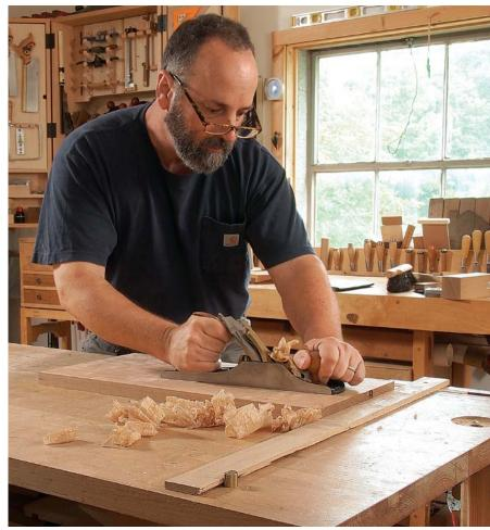
Plane away. The long, low fence offers support all the way across the benchtop without the need to clamp parts in place. Use it to faceplane larger parts and panels (above). In addition, you can edge-plane parts up to 6 in. wide (right).
