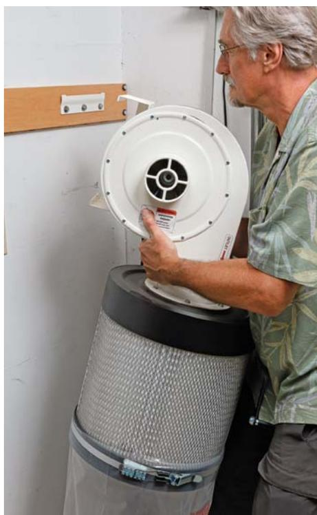
**When floor space is tight.** Though it can weigh about 65 lb., a wall-mounted dust collector can be moved quickly (it just hangs on a bracket) and stored elsewhere if needed. Get an extra wall bracket or two and move it around the shop where it's needed.
