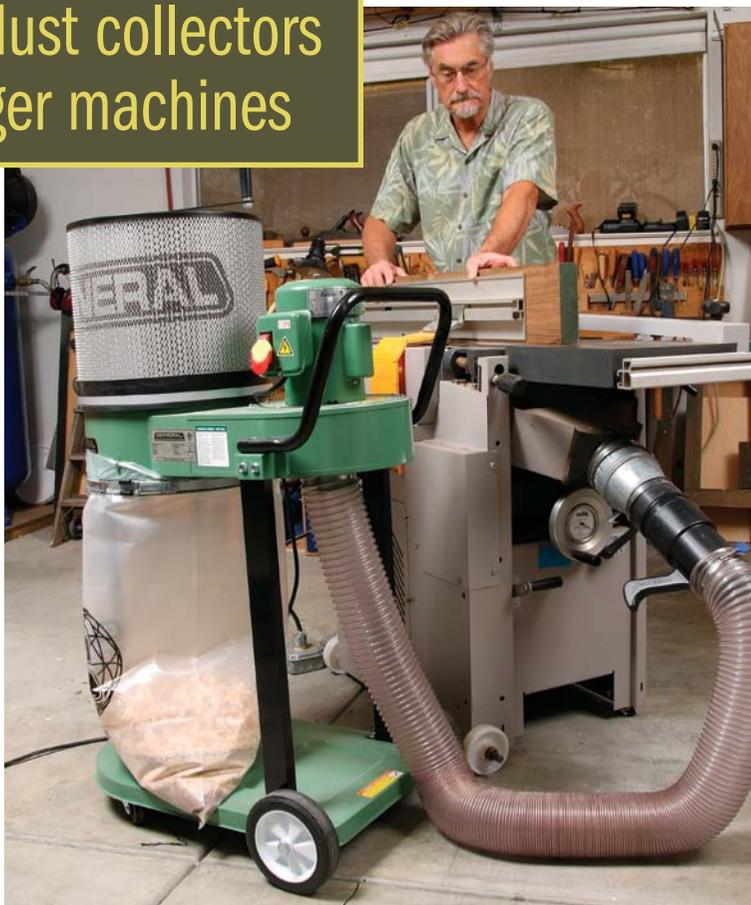
include a jointer and planer. But if your woodworking involves milling rough lumber, a jointer and planer (or a combo machine) are absolutely essential, and so is a dust collector. Jointing and planing wood produces large, heavy sawdust particles, and to move them, a fairly large amount of air volume (about 350 cfm) as well as a 4-in.-dia. hose are required. Shop vacuums aren't suitable for a job that big.
