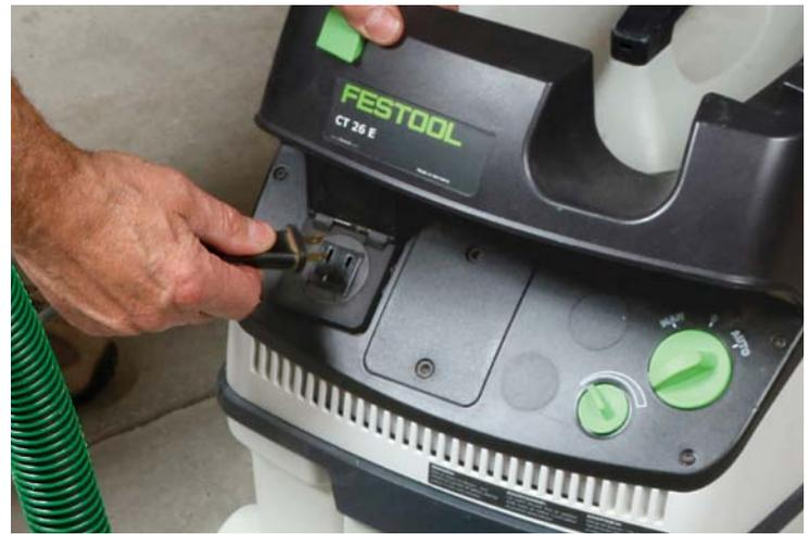
**From a workhorse basic to bells and whistles.** While a sturdy, no-frills model is great to have, a handy feature on higher-priced vacs is the auto-start function. When a power tool plugged into the vacuum is turned on, the vacuum starts automatically.
