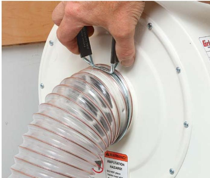
**Toolless clamps and fittings.** Whether they're spring loaded or the thumbscrew type, they're immediately accessible using only your fingers. The thumbscrew type hold a bit tighter than the spring clamps, but the latter are the fastest to get on and off when switching between tools.
