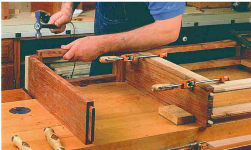
The drawer case is dry-assembled to check that joints fit and to measure for the drawer frames' size. Softwood cauls, hot-glued on the beveled corner blocks, keep clamping pressure in line with the apron tenons. The cauls are chiseled off after final assembly.
