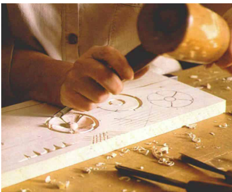
To form the notch between the ends of the petals, Hall makes two converging cuts with a gouge and then pops out the chip between the petals with a third angled cut.
