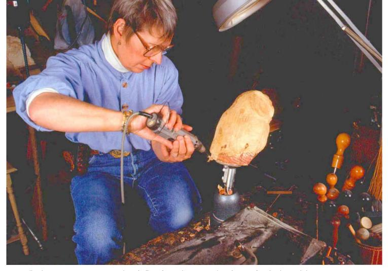
Small, electric power carvers are quick and efficient for roughing out stock and cutting fine details. Bartholomew uses a reciprocating carver to rough out a cedar owl. She will change to a flexible-shaft rotary grinder, like the one hanging by her shoulder, to carve finer details.
