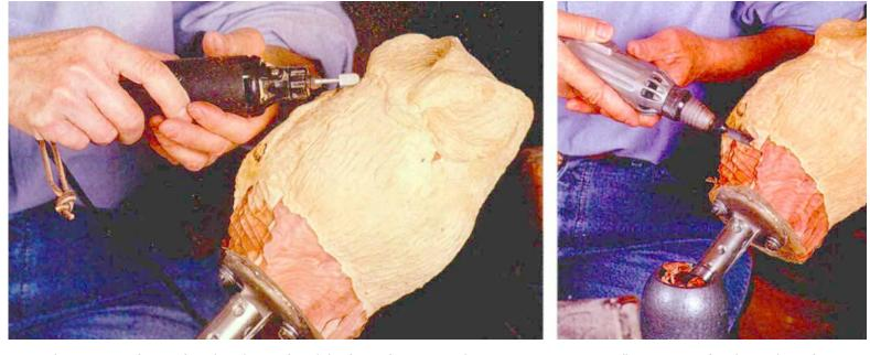
Left: Rotary grinders are fast, but they produce hefty doses of sawdust. The author's two-hand grip makes it easy to control the tool as it cuts: The rear hand holds the tool securely and the front hand guides the cutter as it moves across the cedar blank.
