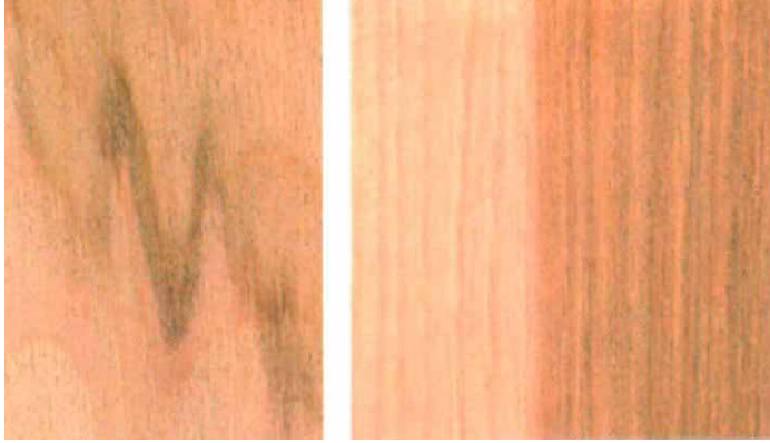
Left: Pecan hickory is commonly darker than true hickory. Its rust-colored heartwood mellows in time to a reddish brown with creamy white sapwood. Right: This sample of true hickory, which is the end scrap of 1-in.-thick by 6-in.-wide tongue-and-groove flooring, is lighter in color than pecan.
