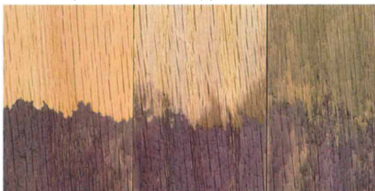
When bleaching iron stains from oak, oxalic acid virtually removes the blue-black stain from the sample (left), returning the wood to its natural color. A/B-type bleach (center sample) leaves the wood more silver, and chlorine bleach (right sample) leaves the wood gray.
