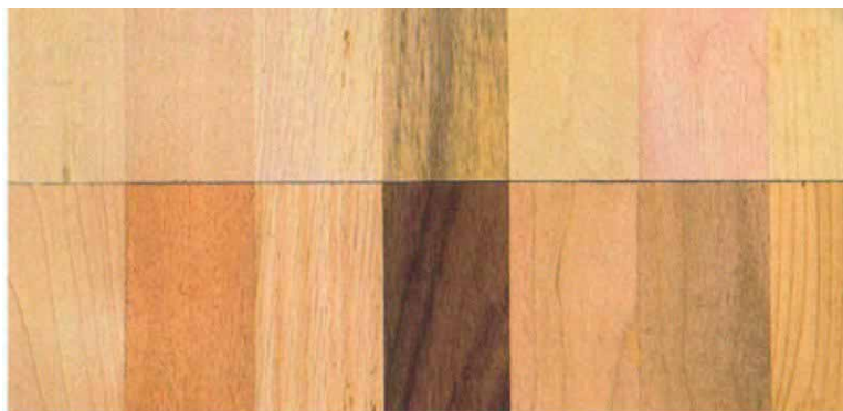
Bleaches react differently to natural chemicals in wood, and even the same bleach has widely ranging effects on different wood species. An A/B wood bleach, applied to the top half of the above samples, had little effect, on the oak and maple (#5 and #7), while it changed the cedar, walnut, cherry, rosewood and mahogany (#1, #2, #3, #4 and #6) more drastically. Although bleached rosewood is lighter, it retains its dark figure lines.
