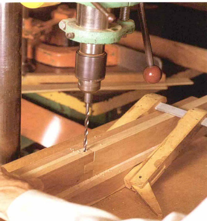
The hinge-pin hole is drilled through the two-part rear apron after an end-to-end finger joint is cut on the two parts, but before the vertical corners are rounded over to form the hinge barrel.
