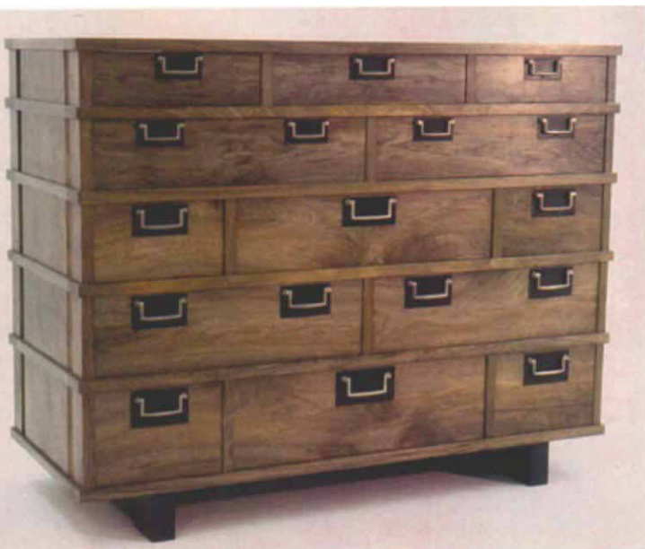
Alan Peters built this chest of drawers in solid English walnut with ebony details. The horizontal frame-and-panel units supporting the drawers allow flexibility for deciding where to divide compartments. The dividers and uprights are doweled into the horizontal units.
