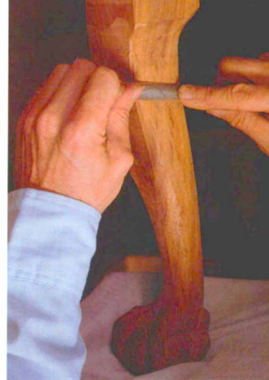
Drawing its teeth perpendicular to the stroke, a mill file leaves the leg ready to be scraped and polished.
