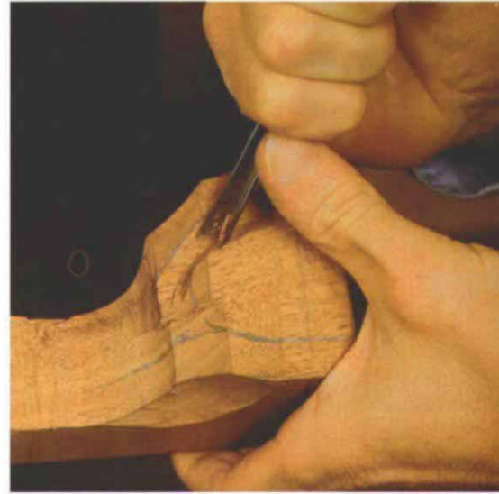
Matching the sweep and width of a 1/2-in.-wide #5 gouge to the original leg (above), Headley cuts the transition from the toe to the ankle accurately (below, left). The outside of the side toe has been scalloped to angle it toward the center toe, forcing the claw to rake back. After marking their width, the toes are roughed out with a parting tool (below, right).
