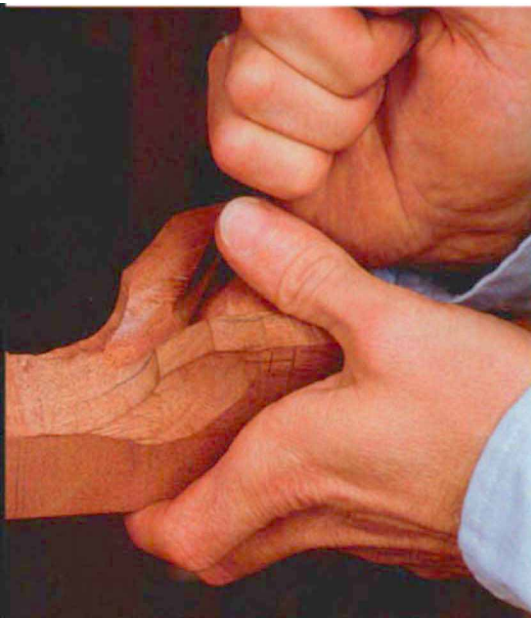
Above: The edge of the web is cut with a 1/2-in. wide #5 gouge. Below: The concave web is cut with a 1/2-in.-wide #5 gouge.
