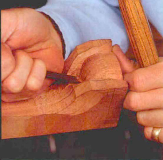
Above: The edge of the web is cut with a 1/2-in. wide #5 gouge. Below: The concave web is cut with a 1/2-in.-wide #5 gouge.
