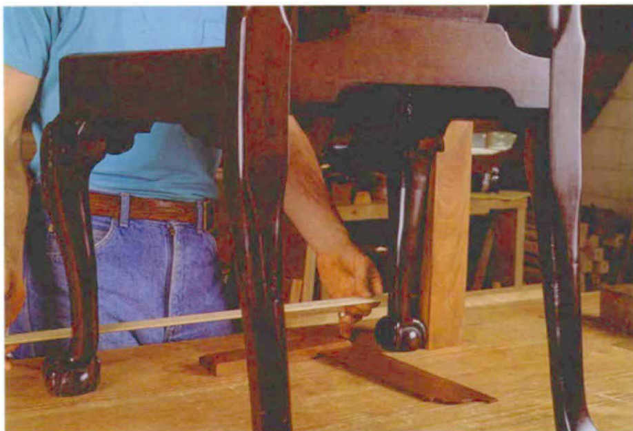
Transfer points from the original leg to the blank following a straightedge held parallel to the floor and against the leg. Mark the blank where the end of the straightedge touches.
