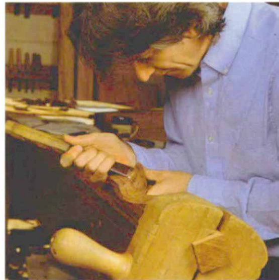
Above: Headley shapes the lower surface of the ball with a 1 1/4-in.-wide #5 gouge, powering the cut with his right hand and guiding it with his left. Right: The author carves across transitional grain at the ball's greatest diameter. The leg is held at a comfortable height and angle in an auxiliary clamp secured in the bench vise.
