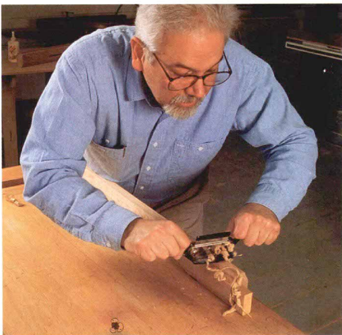
A well-tuned Stanley #80 scraper quickly cleans up bed parts and even makes quick work of cleaning up sawmarks on the chamfers of the cherry bedposts.
