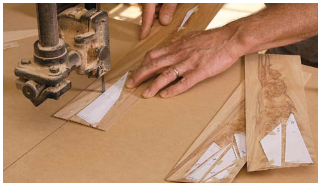
Careful placement. Lamb orients the paper templates to take best advantage of the crotch figure. He keeps an extra copy of the overall drawing and numbers all the parts to guide both grain selection and reassembly.
