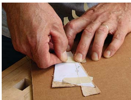
Piece it up. Lamb edge-glues adjacent pieces, clamping them with tape on the show face and the underside. Then he'll cut any joints that cross both pieces.
