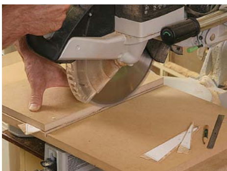
Perfect joints without a knife. After rough-cutting on the bandsaw, Lamb makes finish cuts with a sliding miter saw. His sandwiching jig, made with \frac{3}{4} -in. MDF, keeps the marquetry pieces still and the joint lines perfect.
