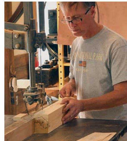
Billets into blanks. After cutting the crotches into billets on the bandsaw mill, then air-drying the billets, Lamb slices the wood into veneers on the bandsaw.
