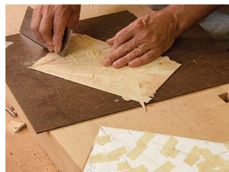
Nearly in the bag. With the marquetry for one quadrant of the design complete, Lamb peels off the tape on the underside, then scrapes the joints flat to prepare for gluing the sheet to a substrate in the vacuum bag.
