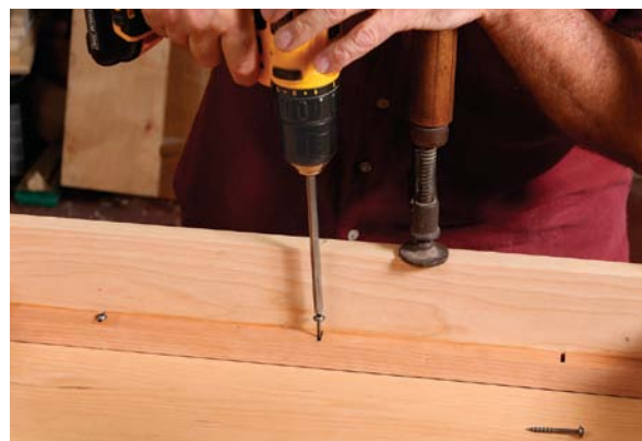
Glue the strips. The ledger strips along the front and back of the table get kerfed at the tablesaw and glued in place about \frac{1}{32} in. from the apron's top edge. The slots in the front and rear strips, as well as the pivoting screws in the side strips, will let the top move without binding.
