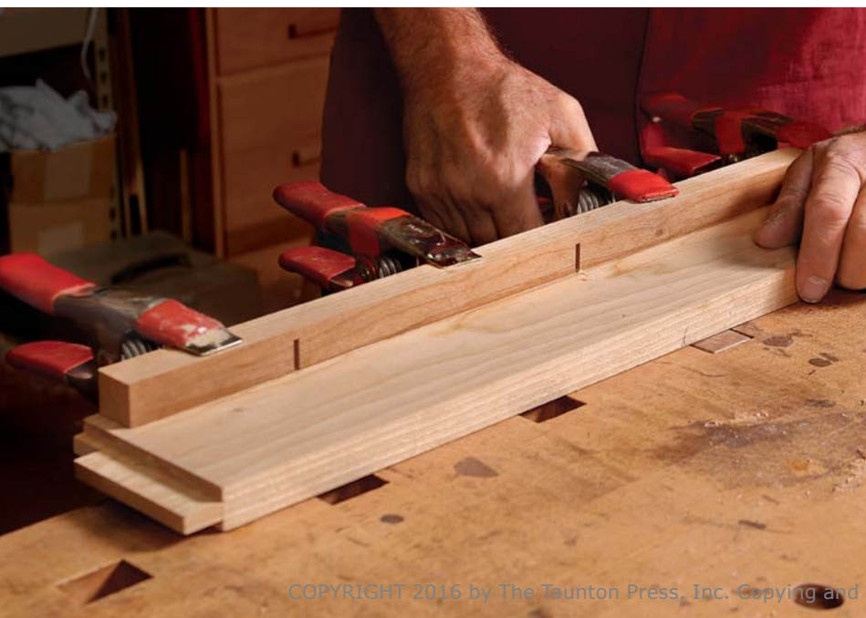
Glue the strips. The ledger strips along the front and back of the table get kerfed at the tablesaw and glued in place about \frac{1}{32} in. from the apron's top edge. The slots in the front and rear strips, as well as the pivoting screws in the side strips, will let the top move without binding.
