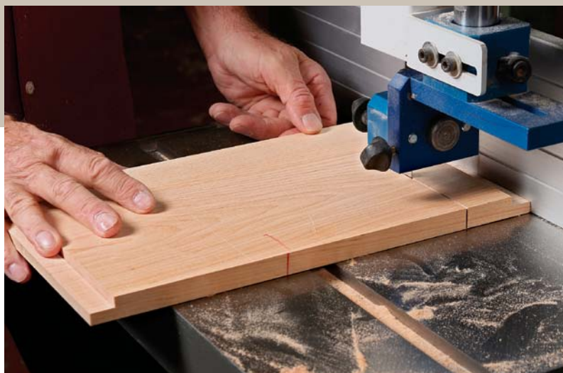
Make some buttons. Cut a rabbet in the end of a flat, wide board and crosscut the buttons to length at the bandsaw. Then move the fence and cut them to width.
