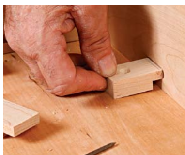
Positioned to allow movement. The buttons will move with the tabletop while keeping it tightly secured. Insert the buttons about halfway into the mortises, then screw them in place.
