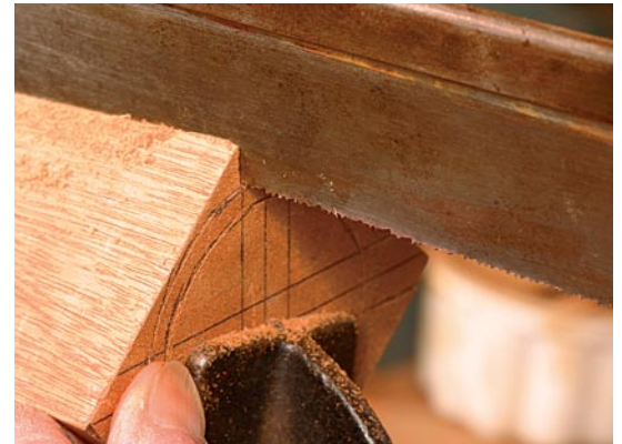
Define the talons. Use a fine-tooth saw to cut just outside the lines marking the width of the talons.
