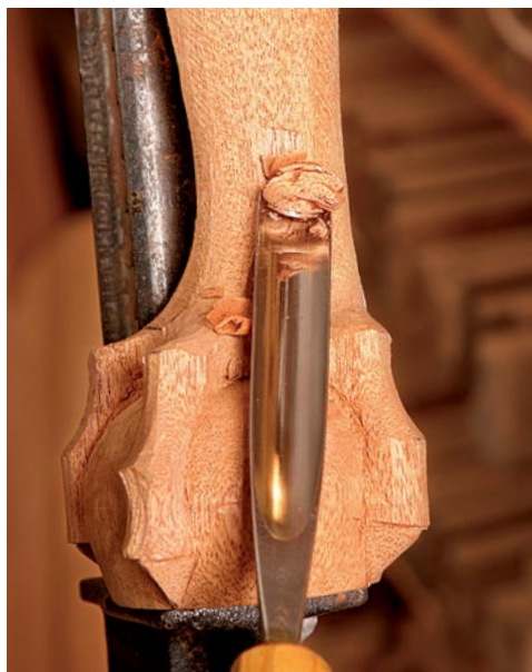
Carve the web. Use a #8-13 mm gouge to hollow out the areas between the center and side talons (left). Work upward from the ball until you feel the wood start to tear, and then make relief cuts downward. Use a #9-7 mm gouge to create the sharp transition from the web into the tendons (above).
