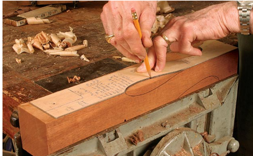
Lay out the leg. Use the template to lay out the cabriole leg on adjacent sides of the blank.
