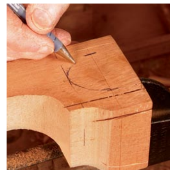
The top of the ball. Extend the lines you drew in the previous step until they reach the break point of the ball. Then draw an arc from these points that connects the midpoint at the top of the ball.
