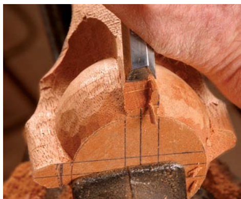
Create the claw profile. Use a chisel to slice downward from the first knuckle to the base of the ball to create a flat, sloping plane.
