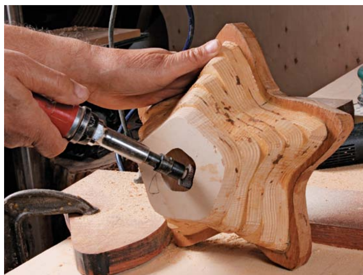
Work in both directions. Leaving the bottom open makes it easier to access all areas of the bowl's interior.
