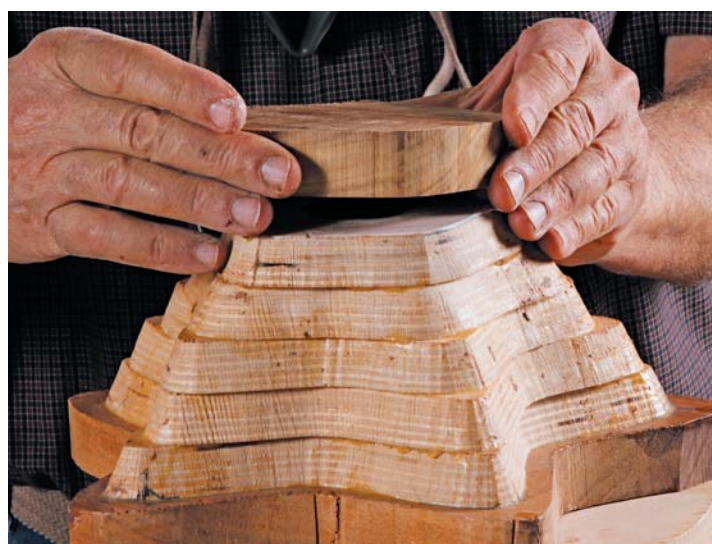
Glue on the bottom. Once the shaping and surfacing of the interior is complete, the bottom gets glued in place.
