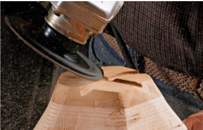
Feet are optional. Vesper uses the edge of a resin disk to quickly give the bowl a four-footed stance.
