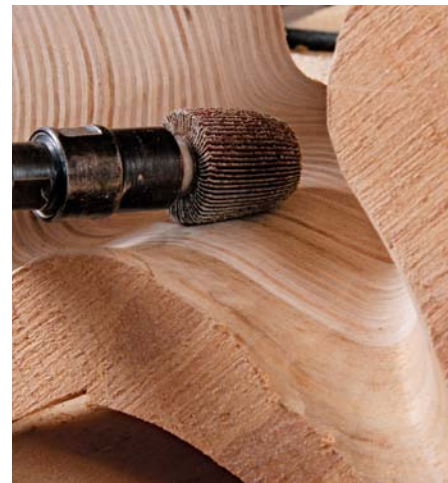
Finish with the flap sander. This narrow attachment refines the surface left by the abrasive cones.
