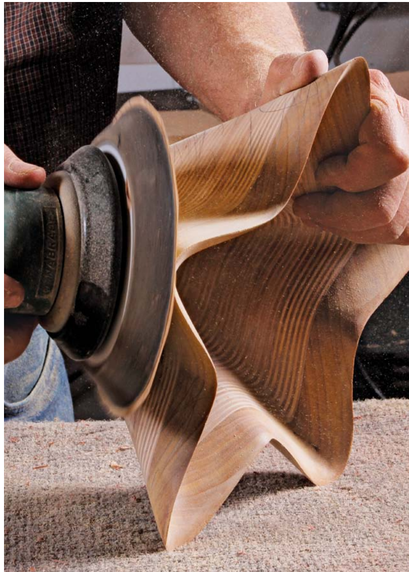
Preparing for finish. A wide flexible sanding pad follows the curves to gently smooth the surface without reshaping it.
