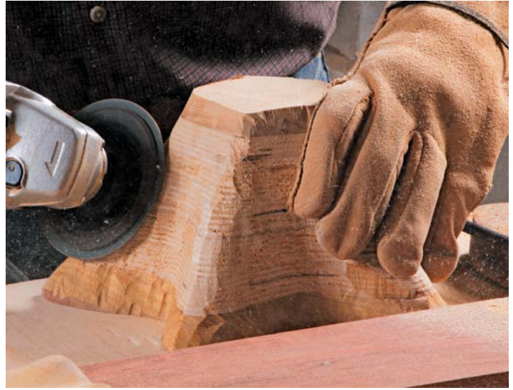
Smooth the transitions. Vesper uses an angle grinder with a resin abrasive disk to refine the shape and smooth the surface.
