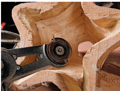
Start with a mini grinder. The tool hogs away material to bring the walls to rough shape.
