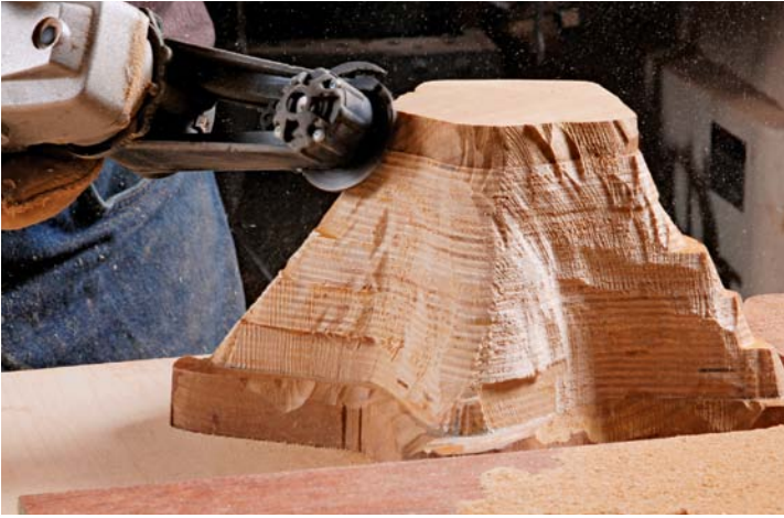
Exterior. The mini grinder once again removes large amounts of stock to rough out the bowl's shape.
