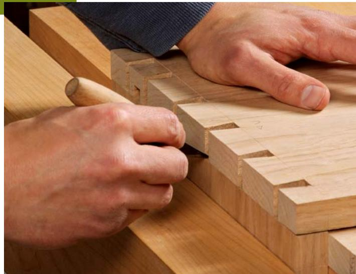
**Now transfer the tails.** You must do this before you miter the tail board, because afterward the mitered tail lacks a surface for registering the knife.
