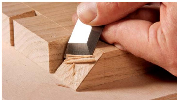
**Saw and pare to the line.** After laying out the miter with a pencil and a combination square, cut just proud of the line (left). Then use a wide chisel to finish the job (above). The slope of the miter should run from the shoulder down to the corner.
