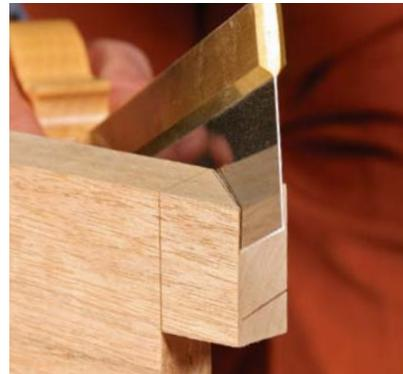
**Two cuts clear the waste.** After cutting the 45° kerf (left), turn the board on edge and saw down the miter (above).
