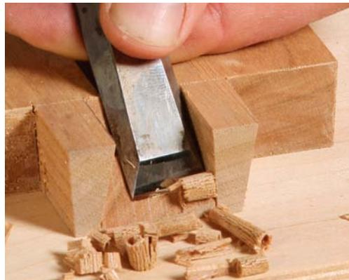
**Pare between the pins.** After removing the bulk of the waste with a chisel and mallet, work carefully to connect the shoulder to the edge of the end grain.
