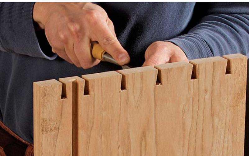
**An important note about laying out the tails.** Use a half tail at the top edges instead of a half pin.
