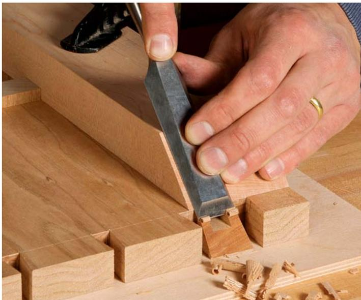
**Here's the place for a guide block.** It can be tough to pare this miter freehand, because there's no pencil line to help. Clamp the block right at the shoulder line and keep the chisel flat on it.
