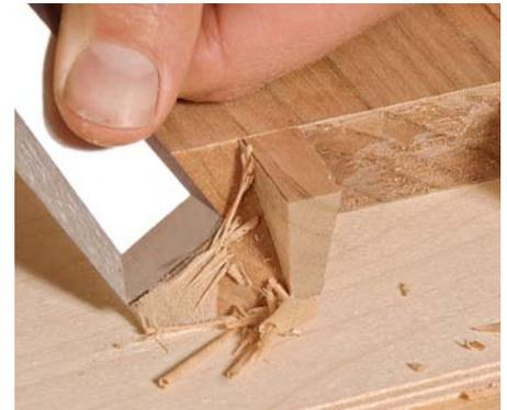
**Clean up the miter.** Work to the shoulder line and the bottom edge of the end grain. The miter will be exactly 45°.
