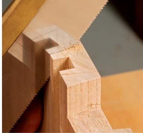
**Make the cuts.** Stop short of the end grain's outside corner, leaving just a bit of waste to pare. This produces a cleaner line on the outside corner when the joint is put together.
