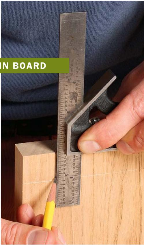
you can wrap the marks you just made down the outside face of the board to the shoulder line. A pencil and square do that job well.
