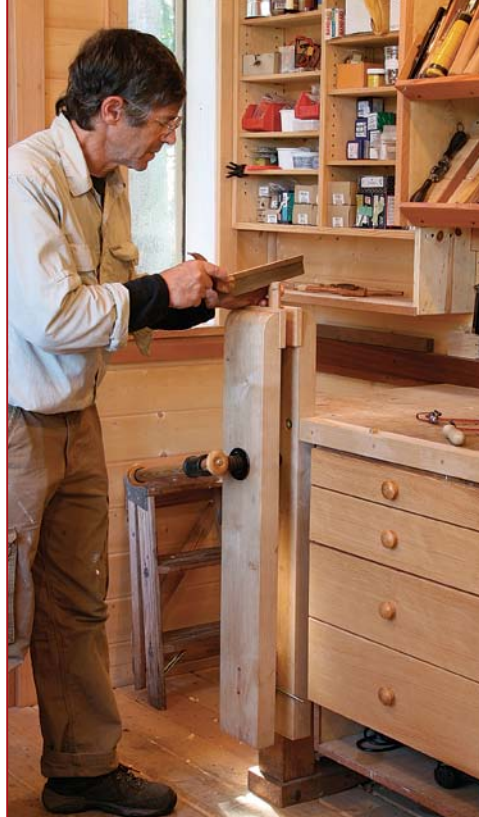
Finer work at a greater height. The tall shoulder vise at Tolpin’s joinery bench brings fine work up close. The benchtop is also elevated to suit joinery work.
