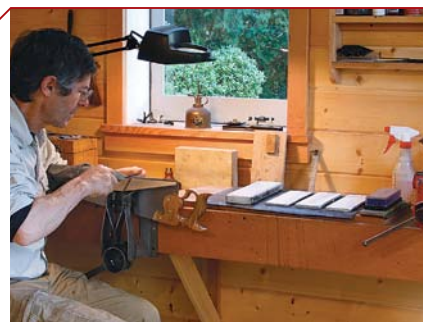
Get sharp. Along with his ceramic stones and diamond plate, which live on a rubber mat, Tolpin’s wall-mounted sharpening bench features a saw-sharpening vise and a task lamp with a magnifying lens.
