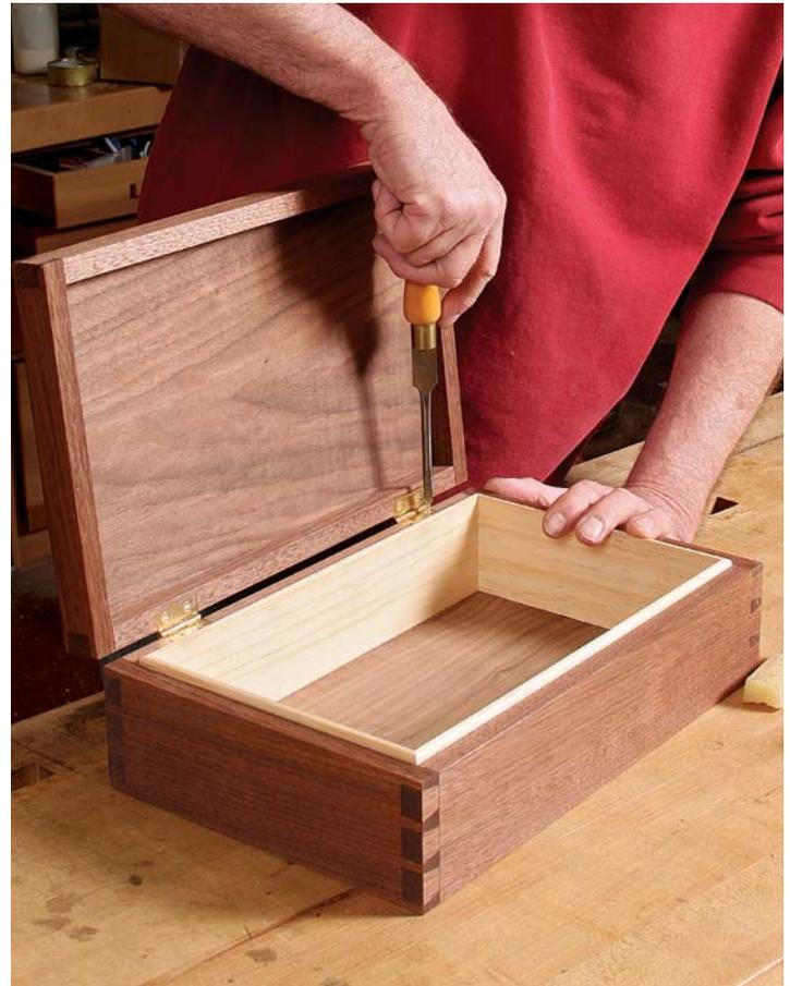
**Hinges and liner.** Brusso brass hinges and a mitered pine liner finish off the box. The liner is held in by a friction fit and left unglued.
