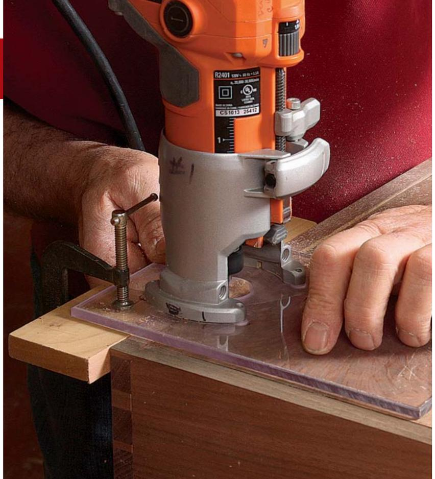
**Keep things square.** Once the routing is done, use a chisel to square up the corners of the groove.
