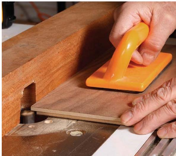
**Rabbet it.** To make the tongue on the panel, you need to cut a rabbet all around. Use a router table and a  $\frac{3}{4}$ -in.-dia. spiral bit for this cut.
