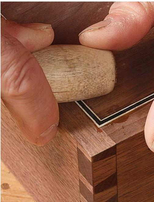
**Burnish and level the banding.** After applying glue to the groove and installing the banding sections, work the belly out of the banding with the back of a chisel (above), smoothing from the center toward each miter. This pressure will close up the miters for a seamless joint. After the glue dries, a card scraper makes quick work of leveling the proud banding with the rest of the box top (right) without harming the book-matched panel.
