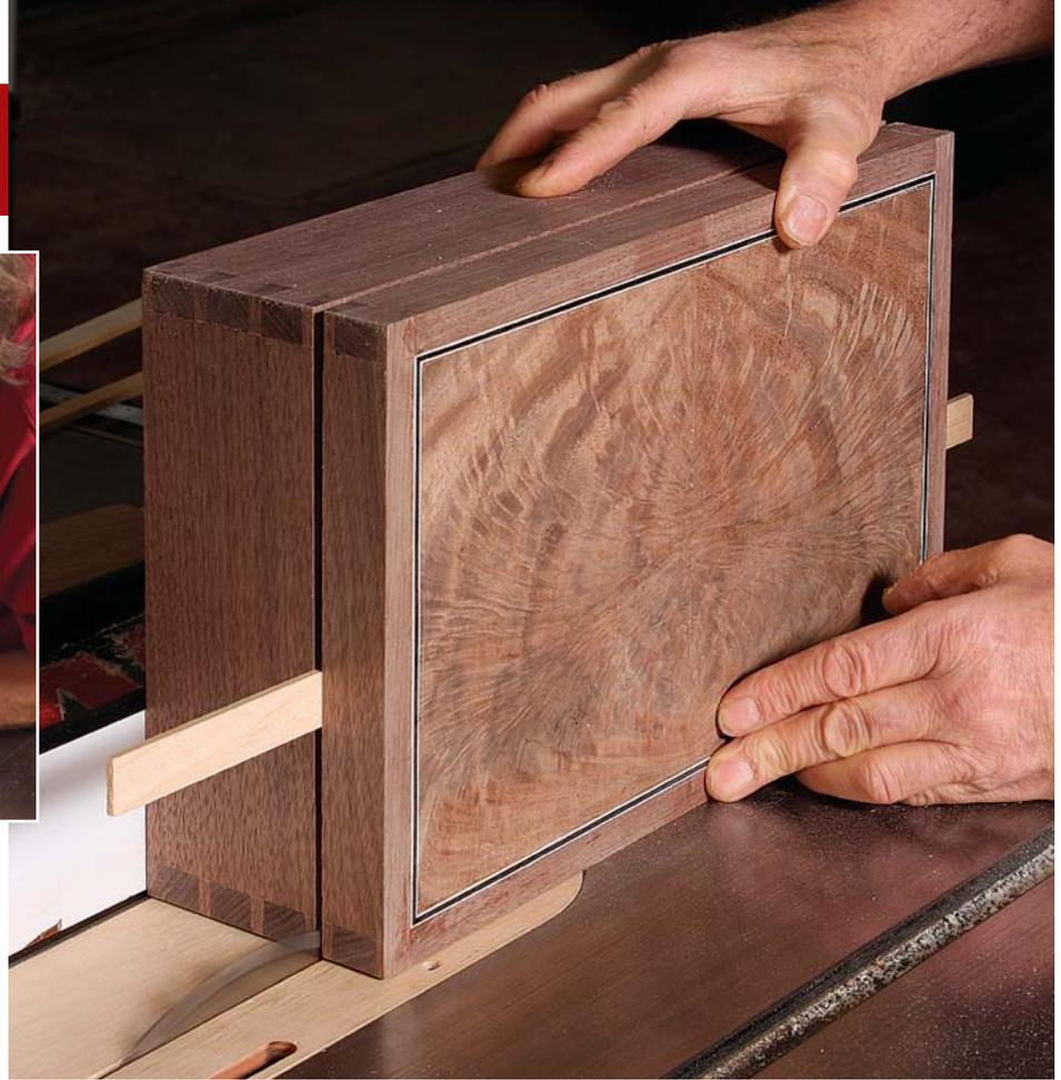
the fence so the blade will cut right in the middle of the wide pin near the top. Before I make the cuts, I make a wood spacer a little longer than the length of the box and a hair thinner than the width of the kerf the sawblade will make.
