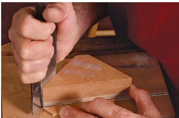
**Simple means of mitering.** A wooden jig allows miters to be cut with a sharp chisel and a steady hand. A wide chisel and a thin strip of wood keep the banding pressed firmly to the block, providing pinpoint accuracy.
