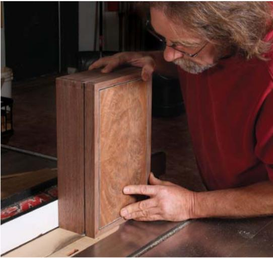
**Off with the top.** Van Dyke prefers using the tablesaw to remove the lid because it leaves behind a clean, square surface (above). Once three of the four sides are sawn, place a spacer whose thickness matches the blade width halfway down (right). Squeeze the top side of the box as it passes the blade. When the cut is complete, the lid will pop off the bottom.
