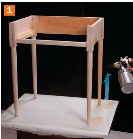
Then spray the outer face in one pass. Masachi starts at the bottom of a leg, goes up and across the apron, then down the other leg with a continuous, smooth motion. Then she returns to the apron to spray any remaining dry spots.
