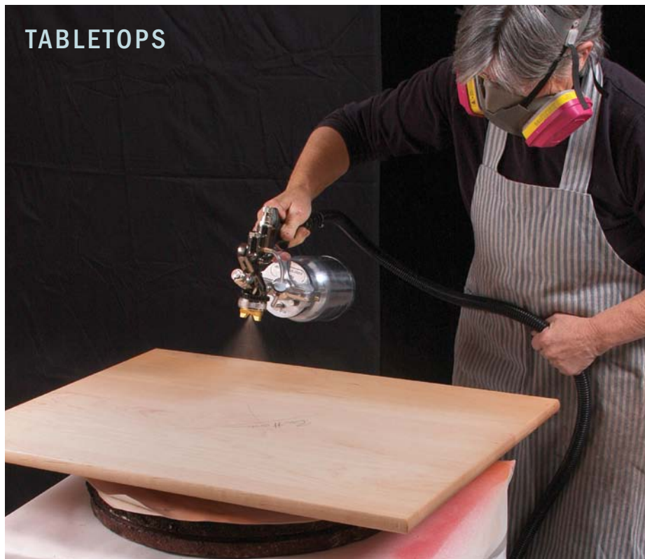
Spray the bottom first. Coat the underside of the tabletop, using a cross-hatch pattern (right) for even coverage. Use a wide spray pattern and overlap each stroke halfway over the last.
