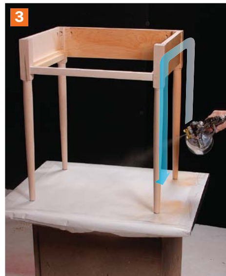
Work one side at a time. Spray the inner surfaces of the legs, using a medium-width spray pattern a little wider than the legs.
