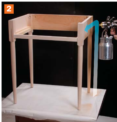
Then spray the outer face in one pass. Masachi starts at the bottom of a leg, goes up and across the apron, then down the other leg with a continuous, smooth motion. Then she returns to the apron to spray any remaining dry spots.
