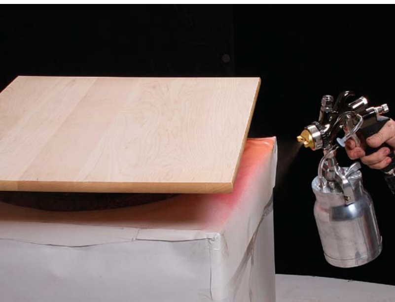
Once dry, flip it over and do the edges. Masaschi dials in a narrow fan pattern for the edges to save material and limit overspray—rogue, partially dried spray particles that can land on other parts of the top, leaving a rough surface on the finish.
