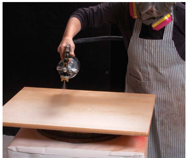
Now spray the top. Because the top is the most visible part of the table, Masaschi does it last to eliminate the chance of getting overspray on it. A smooth finish is most important here, so use the cross-hatch pattern again. Let the top dry before doing the next coat.
