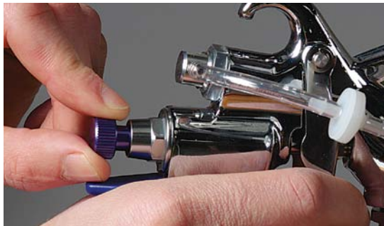
This little knob controls how much fluid you spray. Located behind the trigger, it also serves as the needle's retaining cap.
