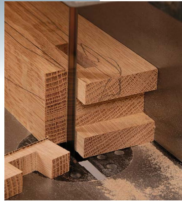
Notch the leg tops for the top rails. Clamp the leg in a tenoning jig and use a dado blade narrower than the notch to cut one face. Rotate the workpiece to finish and center the cut (left). Later, the outside edges of the legs will get tapered, but for now, just notch the top outer edge of each to final width (above) so you can fit the top rails.
