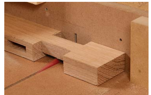
Notch the bottom the same way. Using the same stop blocks as before, lower the blade and cut the bottom of the notch.
