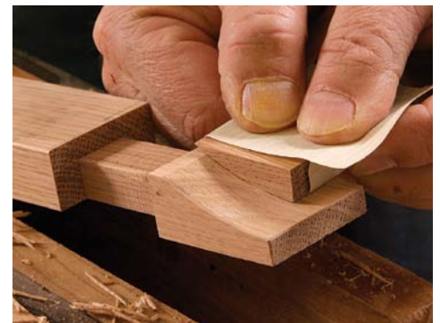
Profile the ends. Cut the cove at the bandsaw, and use the offcut as a sanding block to smooth the shape. Use the first end as a pattern to lay out the remaining ends.
