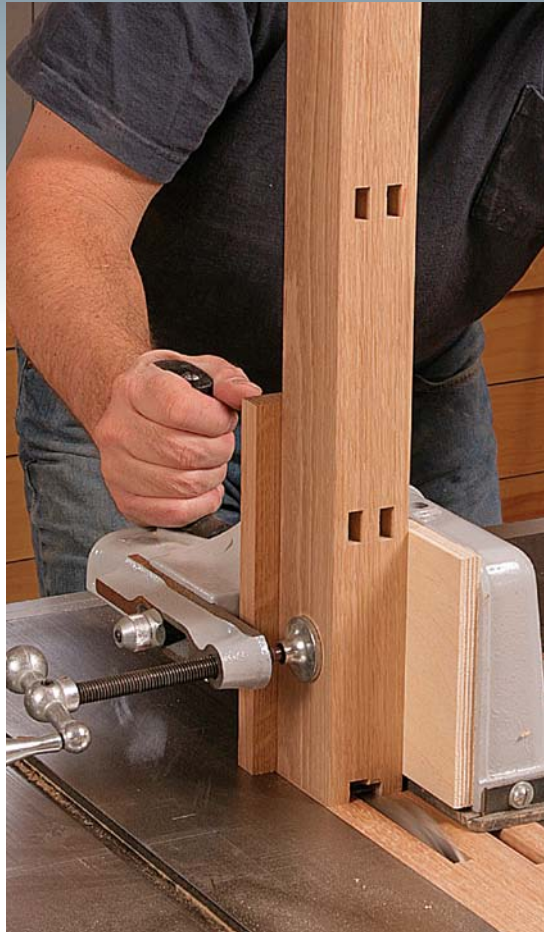
Notch the leg tops for the top rails. Clamp the leg in a tenoning jig and use a dado blade narrower than the notch to cut one face. Rotate the workpiece to finish and center the cut (left). Later, the outside edges of the legs will get tapered, but for now, just notch the top outer edge of each to final width (above) so you can fit the top rails.
