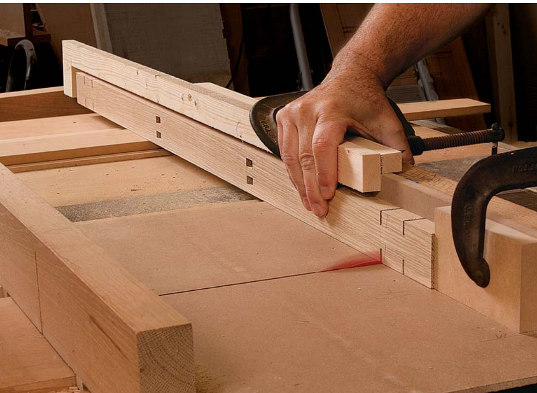
Then notch the rails. Start with the shoulders. Clamp a stop block to the fence for the outside shoulder and attach a hook stop for the inside shoulder (above). Remove most of the waste at the bandsaw, then slide the workpiece across the tablesaw blade to skim off the remaining material.
