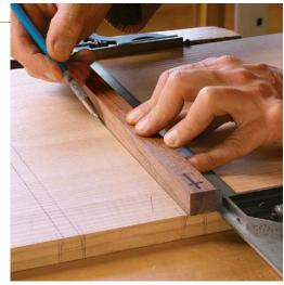
One straight, one tapered. Now that you know the entry point of the top of the bit, extend a square line across the inside face of each case side (left). To mark the tapered edge of the cut (above), use a long wedge that matches the taper, in this case 1/16 in. over 12 in. To avoid confusion, Rousseau boldly marks the fat end of the wedge.
