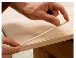
Attach a shim. Lay out the dovetail on the front end of the workpiece, and attach a shim at that edge using double-sided tape. On some dovetails, the shim will go on the back edge.
