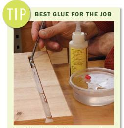
For sliding dovetails, Rousseau prefers Old Brown Glue, a liquid version of hide glue, which is more slippery than yellow glue and offers more working time. Warm the bottle in a hot-water bath to keep the glue thin for use. To create a warm glue dish, pour hot water into a deli container and put the lid on loosely.
