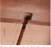
**Setup is easy.** Just align the slot in the fence with the straight side of the slot on the workpiece.
