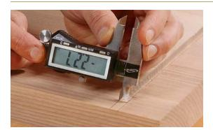
Measure the taper differently. At the open end, you can measure the actual slot. At the other end, you'll need to measure between layout lines, where the mating piece will end. Make the shim accordingly.
