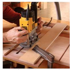
**Rout all of the slots.** Complete each of the slots by routing their tapered edges. Get as close to the pencil line as you can. You'll fit each joint individually.
