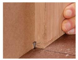
**Use a test piece.** It must be the same thickness and width as the real thing. Rout its tapered side with the shim setup, and then flip the workpiece to rout the straight edge.
