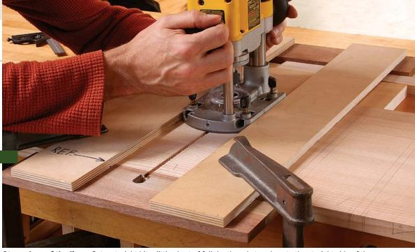
**Steer clear of the lines.** Set a straight bit a little short of full depth and stay close to the straight side of the dovetail slot. Use double-sided tape to attach a straight stick to the front fence to record the path of the cut. Rough out all the slots before switching to the dovetail bit.
