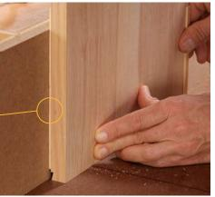
**Creep up on the layout mark by moving the fence.** Then rout all of the workpieces at that setting, attaching the shim where needed. Note the extra stick at the rear to prevent chipout.
