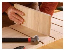
**Start with the widest.** See which slot allows the test piece to slide in farthest, and fit that joint first. Adjust the router until the dovetail goes in all but the last 1½ in. with hand pressure.
