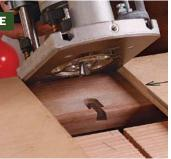
**Change bits.** Insert the dovetail bit and make a cut through the stick attached to the fence.
