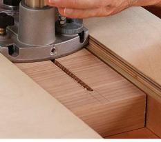
Rout a stopped slot. The three passes are the same, but you'll stop each one at a pencil mark. Square the end of the slot with a chisel.
