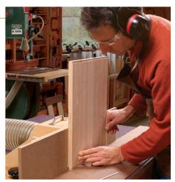
Now the real workpiece. Identify the dovetail that corresponds to that slot, and rout its tapered side. Now follow the same process for the next widest slot, and so on.
