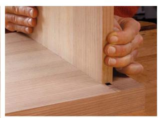
Notch the dovetail and fine-tune the fit. Connect the shoulders with a scribe line (left) and then saw out the notch and pare it flush with the shoulders. Again, hand-fit the dovetails so they slide in about ½ in. short of all the way (above).
