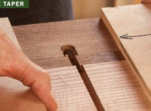
**Same setup trick.** Replace the stick with the wedge, taped to the fence. Rout through it, and use the cut to align the jig with the tapered edge of the slot. Note the slash on the workpiece that indicates the tapered edge of the slot.
