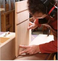
Rout tails the same way. Start with a test piece again, fitting it to each slot individually before routing the real workpieces.
