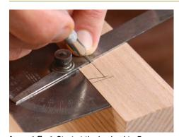
Layout first. Start at the back edge. From there, layout is the same as before, aside from the additional mark for a stopping point.
