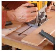
**Rout all of the slots.** As before, wedge a board at the back to prevent blowout.
