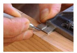
**Outline the slots.** After marking the top and bottom edges of the shelf, mark the width and depth of the slot. Note that each edge of the slot is inset ½ in. from the shelf edges.
