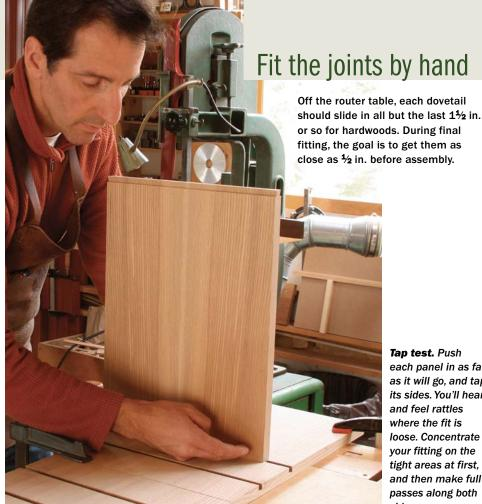
Tap test. Push each panel in as far as it will go, and tap its sides. You'll hear and feel rattles where the fit is loose. Concentrate your fitting on the tight areas at first, and then make full passes along both sides.
