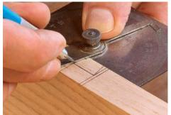
**Angles match bit.** Rousseau uses a 14° bit for sliding dovetails, and lays out the sides of the slots to match.
