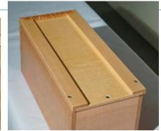
**Drawers without dovetails.** To echo the drawers in traditional Japanese tansu, which are typically nailed or pinned, Levine joined his with small brass screws (left). He built NK-style drawers, which have runners fixed to the bottom. For details on NK drawers, see "A Better Way to Build Drawers," FWW #150.
