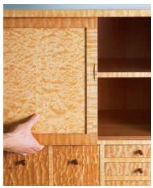
**Out of the bag and into the cabinet.** After sawing the quilted maple veneers for the sliding door panels, Levine glued them to a plywood substrate in a vacuum bag. He also veneered the cabinet top, bottom, sides, and back. The drawer fronts are solid.
