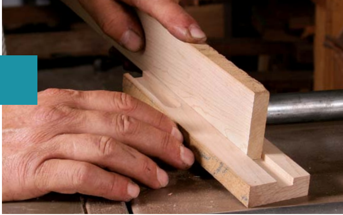
Fit the blank. Make a blank wide enough to produce all the runners you'll need. Plane the blank until it just fits a test groove.
