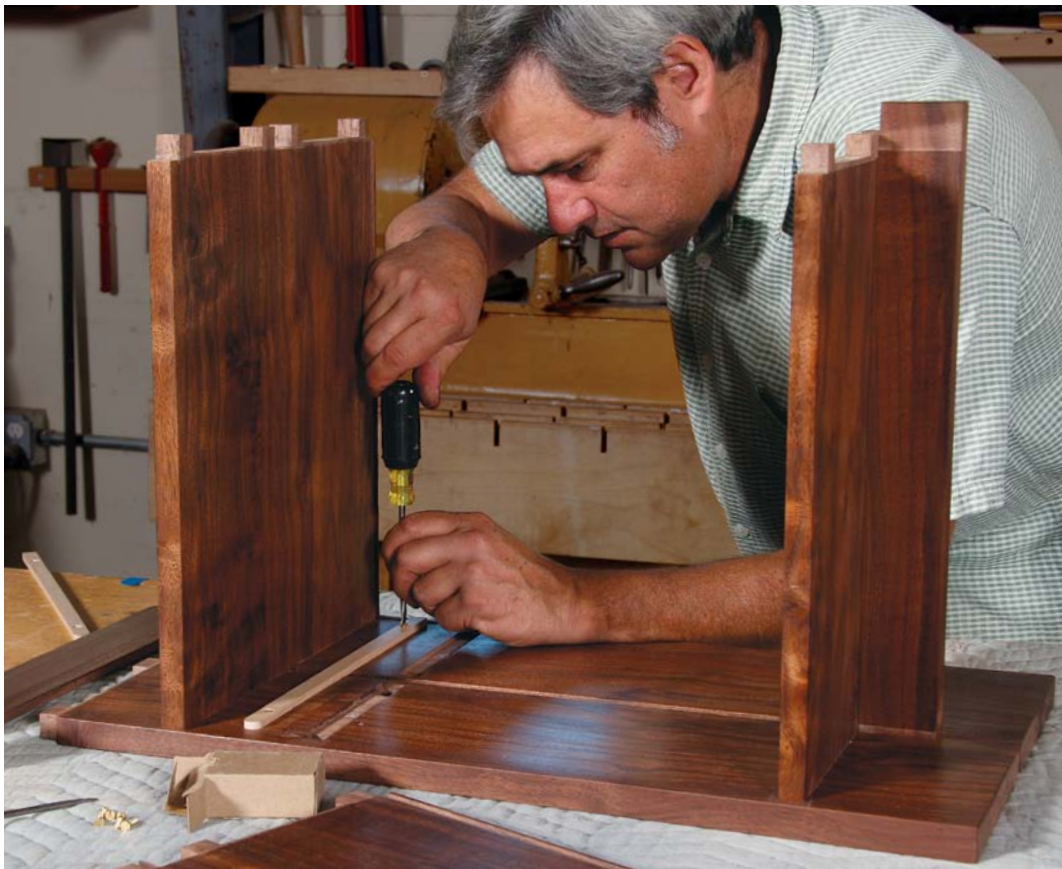
Screwed, not glued. Place the runner in the shallow locating dado in the case side, then fix it with screws. It's good practice to elongate the screw hole in back, for solid cases.
