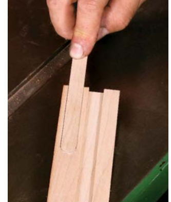
Round the nose. After slicing the blank into runners, sand the leading end round to match the end of the groove. Check the fit with a stopped test groove.
