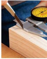
Measure or mark. The step lets you use the end of the jaws as a depth stop of sorts, for measuring distances (left). You can also slide the tool along an edge for marking and scribing (right).
