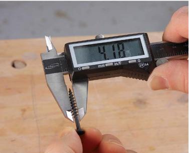
Pilot and clearance holes. Use the skinny part of the jaws to reach between the threads and measure the central section, called the root (above). Use the flat part of the jaws to measure the outside of the threads (left).
