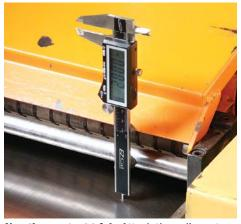
Use the magnet trick. Attach the calipers to your planer with magnets, so you can adjust the bed precisely for the final pass.
