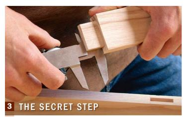
Square and steady. The step on the back of the sliding jaw is often overlooked. It registers squarely against the edge of a workpiece while the end of the tool is used for measuring.
