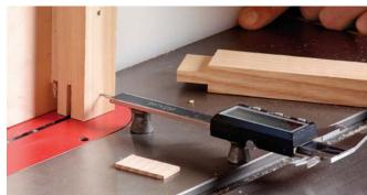
Add magnets and make machines digital. Use these standoff magnets from Lee Valley (leevalley.com) to attach calipers to a metal surface, and then use the depth rod to make precise adjustments to fences, jigs, and more
