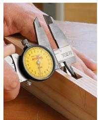
Inside for width. Use the inside jaws to find out exactly how wide a mortise is before cutting the tenon. They are also great for positioning a jig on a workpiece, and dozens of other
