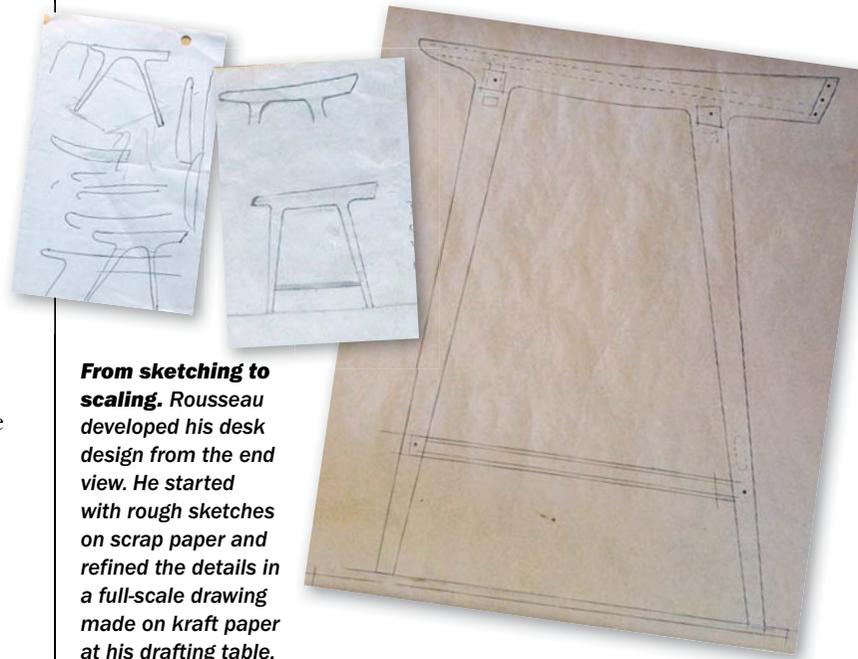
**From sketching to scaling.** Rousseau developed his desk design from the end view. He started with rough sketches on scrap paper and refined the details in a full-scale drawing made on kraft paper at his drafting table.
