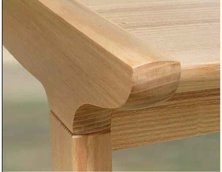
**Slight curves soften the surfaces.** A shallow curved profile routed onto some parts softens their look and feel without losing the hard arrises that provide visual definition. In a detail borrowed from Danish Modern chairs, Rousseau used a small chamfer where the leg meets the end cap; it defines the joint and makes fitting it less exacting.
