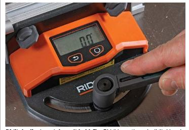
**Digital adjustment doesn't hold.** The Ridgid was the only digital head tested, sacrificing detents for adjustability to  $\frac{1}{10}$ °. While getting an angle is easy, tightening the handle causes the gauge to lose its setting.
