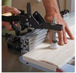
Hold-down for long crosscuts. A long board hanging off the table can be hard to control safely as you cut it. JDS offers a clamp-down accessory \$59) with its Accu-Miter gauge that keeps the stock firmly on the table.
