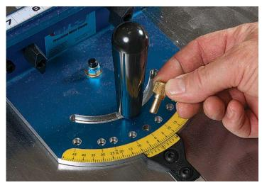
**How to handle in-between angles.** The Kreg uses a brass pin to lock in common angles. When operating outside these angles, the vernier scale allows accurate adjustments down to  $\frac{1}{10}$ °.
