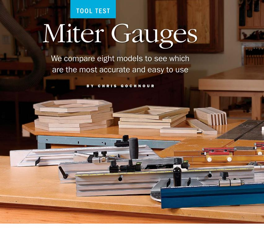
great tablesaw setup should include a great miter gauge as part of the package. This important accessory ensures safe, accurate crosscuts on boards and small panels and is great for joinery cuts, too. Unfortunately, the gauges provided with most new tablesaws often are less than ideal, with play in the miter-slot fit that can't be tuned, a head that's hard to read and set, and a fence that's too small (or nonexistent) to support your work.
