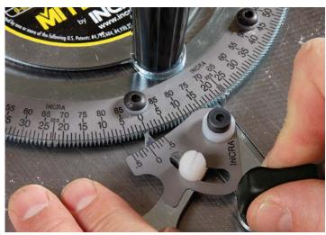
**Detents for every angle.** The Incra 1000 HD has positive detents every  $1^{\circ}$  of its range and at  $22.5^{\circ}$ . This is a perfect medium between the 1000 SE's too-broad  $5^{\circ}$  increments and the 3000 SE's tedious  $\frac{1}{2}^{\circ}$  increments.
