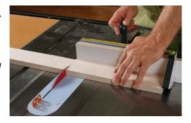
Miter test. To test the accuracy of miter cuts. flip-stops, and head settings. Gochnour made picture frames. An accurate gauge will cut equal-length pieces.
