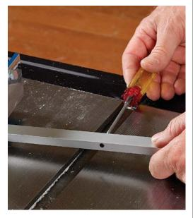
test, the octagon test, and the long stock test. The straight-cut test ensured the 0° setting on the head was perpendicular to the blade. I used each gauge to cut a piece of poplar roughly in half, then I placed the halves edge-down on the tablesaw and flipped one over. Flipping the piece doubles any error in the cut and exaggerates how off the gauge is.
