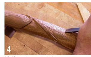
Climbing ivy. Brown carved the ivy before final glue-up so that the parts could be worked on dry-assembled or separated. He drew the leaves freehand, but used an old carver's trick to establish a natural-looking line for the stem, winding string around the parts and tracing it.
