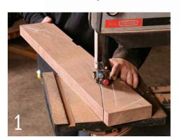
**Join, then saw.** Brown cut the mortise-andtenon joints while the blanks were still square, then bandsawed out the legs.
