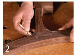
**Chamfer layout.** The shaping will begin with chamfers chiseled along the length of the parts. Here, with a leg and stretcher dry-fitted, Brown lays out lines to guide the chamfering.
