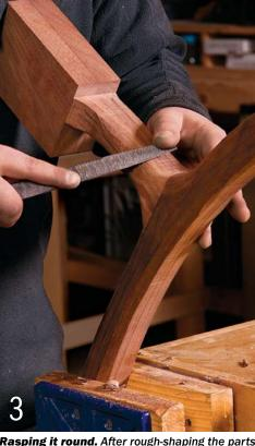
Rasping it round. After rough-shaping the parts with chamfers, Brown refines them with a rasp. Because the parts swell at the junction to mimic branching, he added gunstock miters to the mortise-and-tenon joints to avoid problems with short grain.
