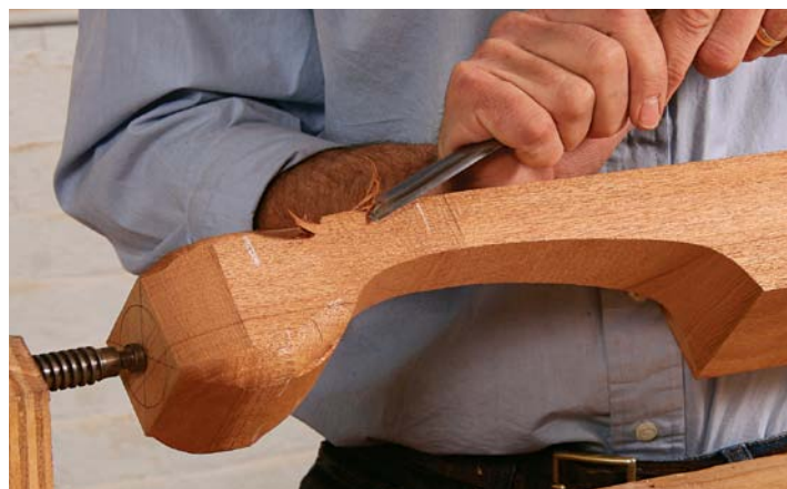
Incurve at the ankle. The rear claw has an inward curve that begins above its one knuckle. Create the curve with a #7-20mm gouge, making cuts from the bottom and top that meet in the middle. Alternatively, this curve can be shaped with a rasp or a spokeshave.
