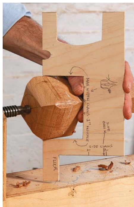
Chamfer and check. Using a #7-20mm gouge, knock off the corners of the foot until the gouge fits over them.
