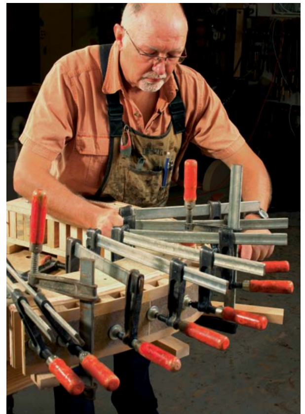
All in a row. It is best to work with the form lying down. Start at one end and work clamp by clamp toward the other end, using a stand to support all the plies and parts, especially at the beginning.
