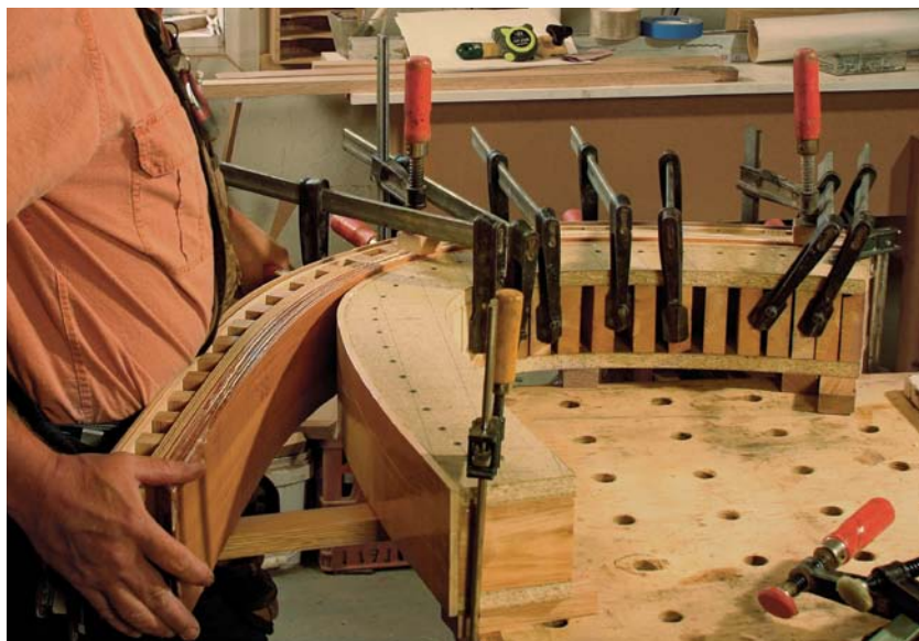
Lots more clamps. It took 20 F-style clamps to complete this glue-up. Note the additional sideways clamps over the posts that keep the plies aligned.
