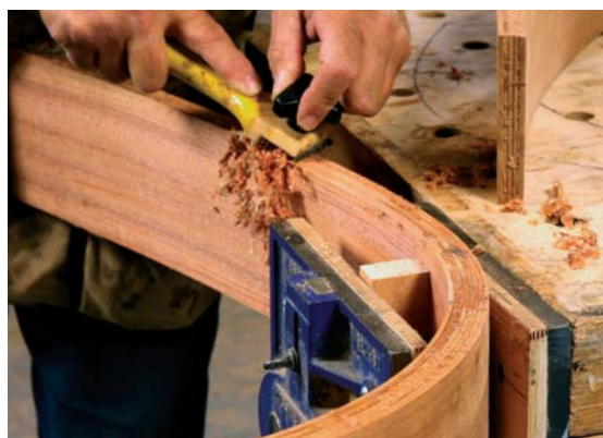
Scrape away squeeze-out. Fortune uses a paint scraper, sharpened on the bench grinder, to scrape all the hardened glue off the edge that will be jointed.
