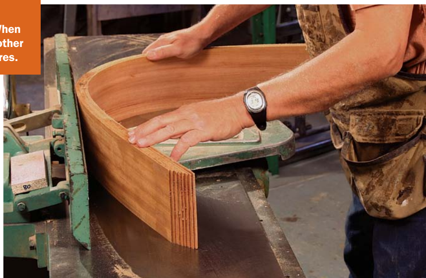
Joint one edge. Curved pieces are easy to joint. Just move the piece in an arc so the area being milled stays at a right angle to the cutterhead. After jointing the arms, place them back on the form and transfer the mark for the floor level. That will help you in Part 2.
