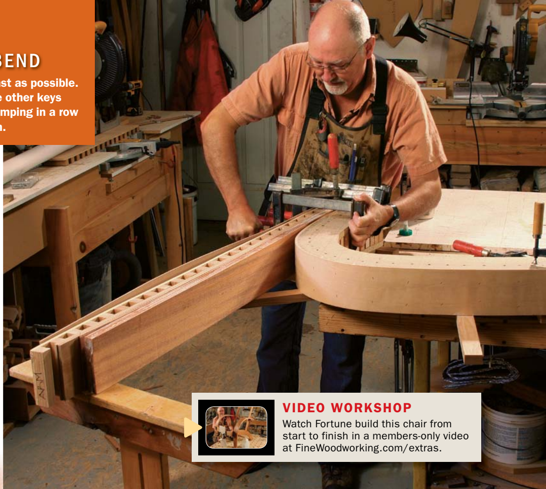
All in a row. It is best to work with the form lying down. Start at one end and work clamp by clamp toward the other end, using a stand to support all the plies and parts, especially at the beginning.
