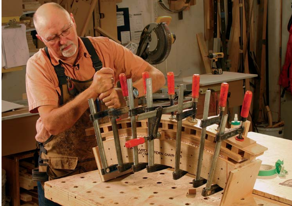
Slat form sits upright. The seat and back slats on this outdoor chair have a shallow curve. So Fortune attaches legs to the form and stands it upright. That means it is easier to start clamping in the center in this case, and work toward both ends.
