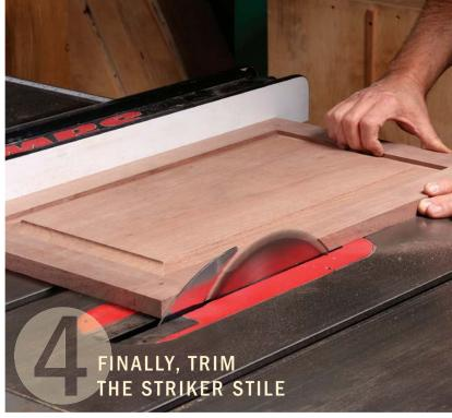
**Make a trimming cut.** Rip off as much of the excess as you dare, while the door is still separate from the cabinet.
