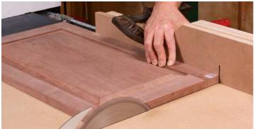
**Trim for a perfect fit.** Take off just enough to get this edge into the cabinet, and then recheck the fit, with the shims at the bottom. If you find a tapered gap at the top of the door, use a shim to taper the next cut. Go for the same even, ½-in.-plus gap. Sand or plane off the sawmarks.
