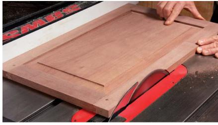
First cut is the deepest. If the door opening is relatively square, take a full 1/8 in. off the hinge stile now (left). If not, trim off less. Remove sawmarks with a handplane (below).
