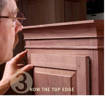
**Check it first.** Hold the hinge stile tight to the cabinet again, but this time set the door on ½2-in. shims to create the proper gap at the bottom.
