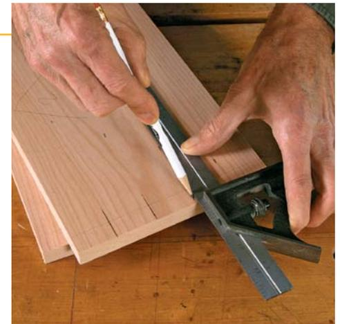
**Transference.** Use a square to transfer the center marks of the pin sockets to the end of the board.
