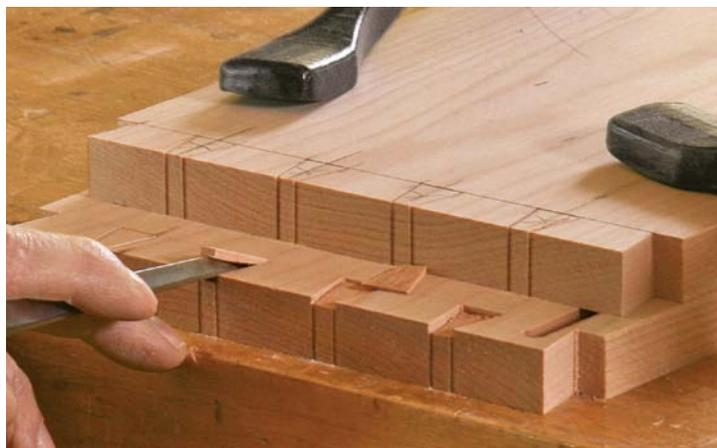
**Pop out a slim chip.** After lightly chopping all the pin sockets, use a narrower chisel to remove the top layer of waste wood with a tap into the end grain. The shoulder should now be about  $\frac{1}{16}$  in. high.
