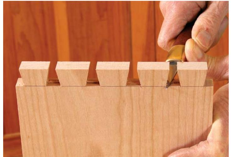
**Knife work.** Use a sharp knife with a narrow blade to clean up the tight corners of the pin sockets.
