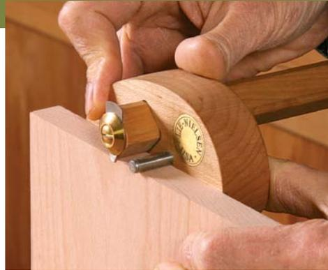
**Set the gauge.** Adjust the marking gauge so its cutter just overhangs the pin board (above). The overhang will produce dovetails that are slightly proud. Scribe the baseline across both faces of the tail boards (right).
