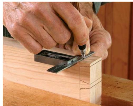
**Reclamp and re-mark.** To mark and cut the shoulders of the half-pin sockets, turn the tail boards 90° in the vise, being sure to keep all sides flush.
