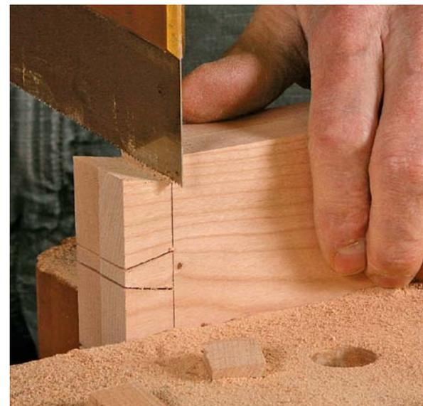
**Make it easy on yourself.** Repositioning the boards is worth the trouble, since a vertical cut is much easier to make accurately.
