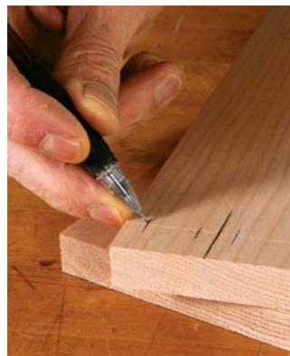
**Chisel trick.** Establish the width of the pin sockets by tracing the chisel you'll use to chop them. Using a fine pencil, mark across the scribe line on each side of the chisel (above left). Gauging by eye, make a mark for each of the half-pin sockets so they are roughly half the width of the full-pin sockets (above right).
