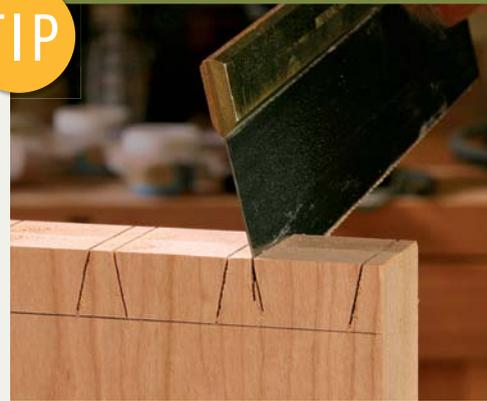
**Oops.** If your cut wanders far off track, start a new kerf parallel to the original pencil line. One of the tails will be slightly narrower than the others, but the angles will be consistent.
