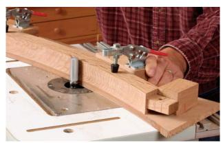
**Easier pattern mounting.** At a router table, a pattern bit lets you clamp a workpiece to the top of a pattern (above), which makes it faster to shape multiples. For handheld routing, the pattern must be secured to the top of the workpiece (right).
