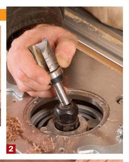
jobs where you need a perfect surface with two clean corners, like when working with veneer, compression spiral bits really deliver. Their cutting action pulls fibers toward the center for a clean edge top to bottom. These bits also excel when cutting extra-brittle solid woods where both corners won't hold together with spiral bits.
