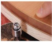
Tame tearout on veneer. A spiral bit leaves chipout on the lower edge of a veneered panel (top). Cutting the same piece with a compression bit, however, yields a perfect cut with no chipping on either edge (bottom).
