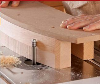
Tag team for wide parts. With the template on the bottom, rout the lower portion of the stock with a pattern bit (left). Then flip the workpiece and finish routing with a flush-trimming bit, registering the bearing against the previously routed surface (above).
