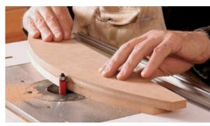
**Shop workhorse.** Inexpensive straight bits are great for MDF and plywood, which can wear out a bit quickly.
