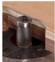
trimming bit works great for most types of routing projects, and because it is safer, it's usually my first choice for both the handheld router and the router table. For the projects that a flush-trimming bit can't handle, a pattern bit fits the bill.
