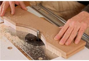
**Good for handheld and router-table tasks.** On a router table, mount the pattern on top of the workpiece (above). For handheld routing, the pattern must be attached to the bottom (right).
