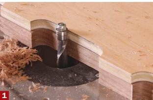
Rout halfway and flip. Start with the template on top and use a flush-trimming bit to rout half of the profile working downhill (1). Then install a pattern bit (2) and flip the workpiece and template to rout the remainder of the profile (3).
