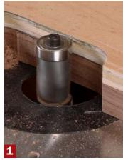
The steps are the same as before, but you'll finish in less time. Start with the top bearing aligned to the pattern (1). Instead of changing bits, simply raise the bit to align the bottom bearing with the template (2) and finish routing the profile (3).
