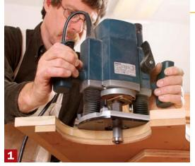
Bring the router to the work. On projects too big for the router table, start routing with the template on the bottom (1). Then flip over the workpiece (2), extend the bit, and finish the job (3).
