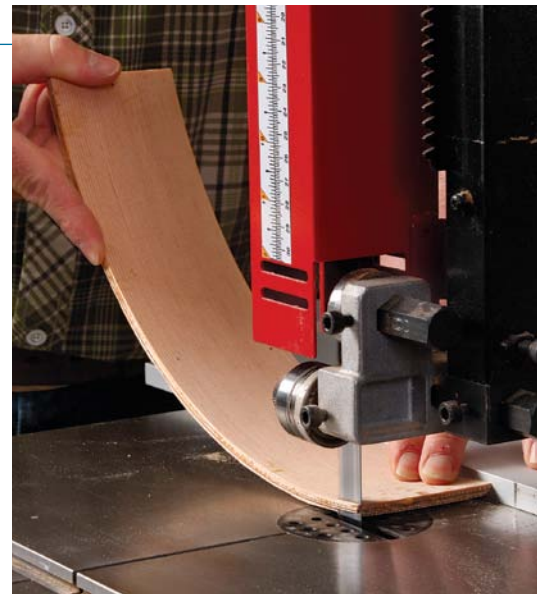
Start at the bandsaw. Resaw the plies for the drawer fronts at \frac{1}{16} in. thick (left). Joint the face of the board after each cut. Secure the blank with two nails (center), cover with a caul, and pull the ends down with packing tape. After jointing one edge of the glued-up blank, trim the blank to width at the bandsaw (right).
