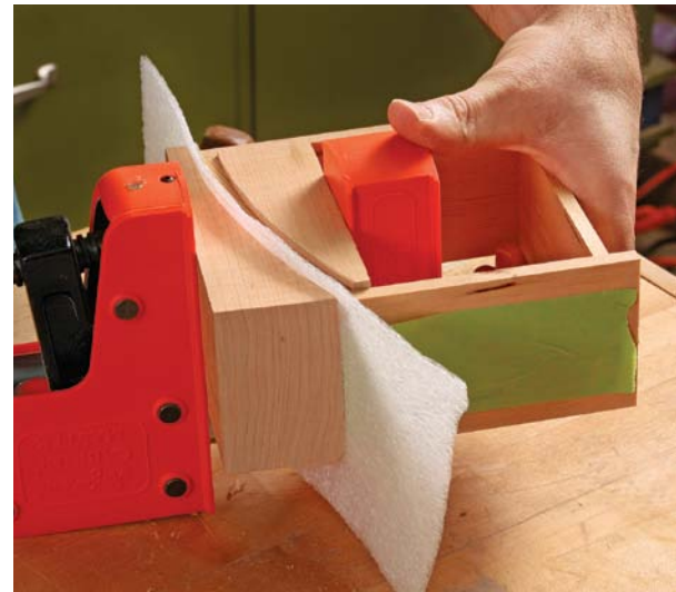
Attach braces and apply clamping pressure. A couple of pieces of thin stock backed with double-sided tape prevent the drawer front from pivoting as the clamp tightens.
