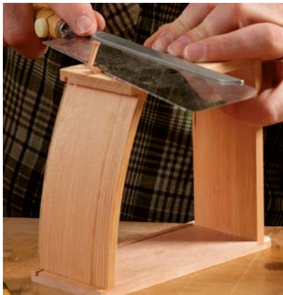
Pegs reinforce the joint. Kenney seats three shopmade pegs in holes drilled on each side, then trims them flush with a pull saw and chisel.
