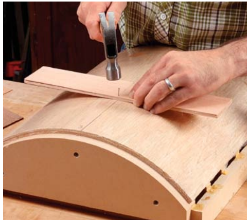
Start at the bandsaw. Resaw the plies for the drawer fronts at \frac{1}{16} in. thick (left). Joint the face of the board after each cut. Secure the blank with two nails (center), cover with a caul, and pull the ends down with packing tape. After jointing one edge of the glued-up blank, trim the blank to width at the bandsaw (right).
