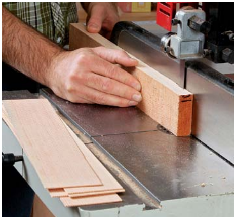
Start at the bandsaw. Resaw the plies for the drawer fronts at \frac{1}{16} in. thick (left). Joint the face of the board after each cut. Secure the blank with two nails (center), cover with a caul, and pull the ends down with packing tape. After jointing one edge of the glued-up blank, trim the blank to width at the bandsaw (right).
