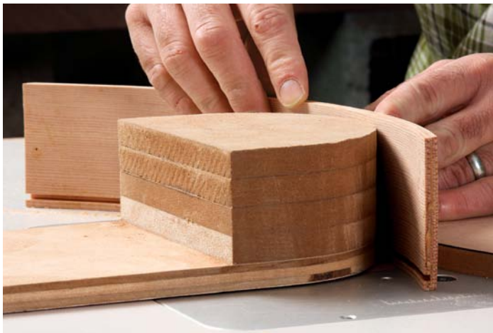
Final touches. A curved fence at the router table makes it easy to cut the groove for the drawer bottom (above). At the tablesaw, a curved auxiliary fence for the miter gauge holds the workpiece securely and ensures that the end grain is cut at the correct angle (right).
