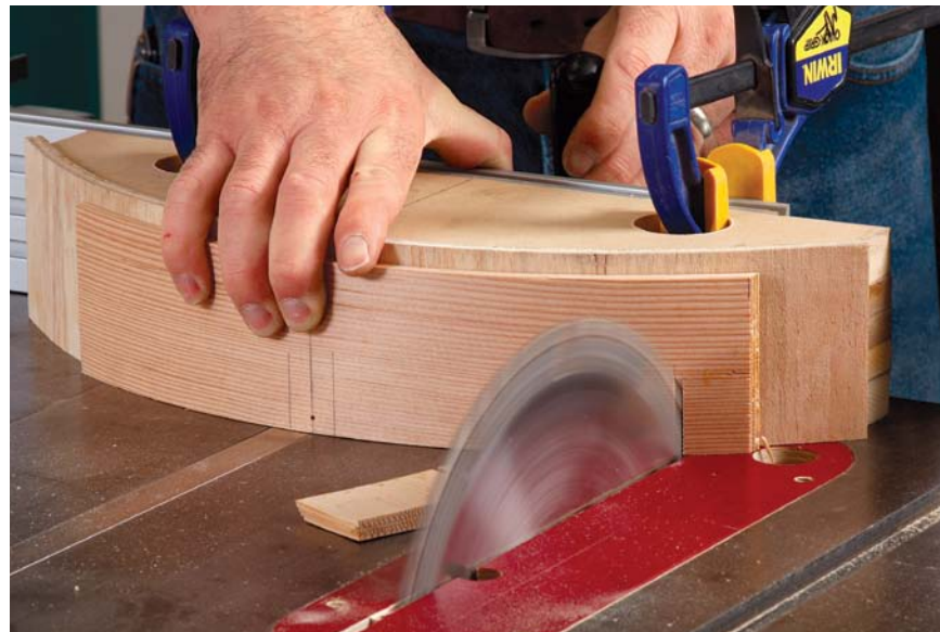
Final touches. A curved fence at the router table makes it easy to cut the groove for the drawer bottom (above). At the tablesaw, a curved auxiliary fence for the miter gauge holds the workpiece securely and ensures that the end grain is cut at the correct angle (right).
