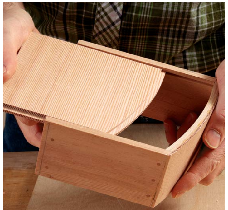
Install the bottom. The curve on the bottom's front edge (below) is cut at the bandsaw after tracing the profile from the glued-up drawer.
