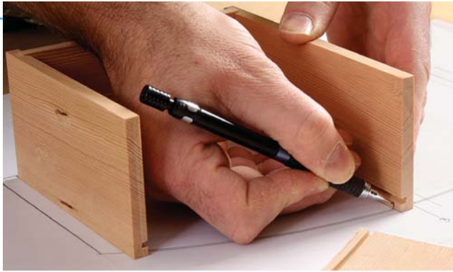
Mark the front's location. Working from a full-size drawing, mark the drawer sides for the location of the drawer front.
