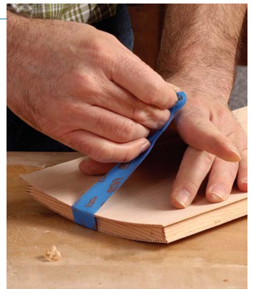
Bandings before veneers. Glue on the solid-stock top and bottom bandings, then trim them flush at the router table (left). Fit the door to the case vertically, and then add the side bandings (center). The veneers on the front and rear faces (right), are glued up separately in the vacuum bag.
