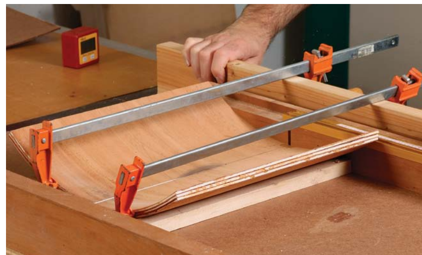
Rip the panel in half. With the trimmed end against the sled's fence, Kenney centers the panel on the sled's kerf and rips it in half. A loose batten on either side keeps the piece from rocking.
