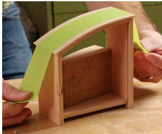
Attach the face veneer. Painter's tape holds the veneer in place (above) until the glue-up is secured with clamps and shaped cauls (right). Thin packing foam helps distribute the pressure.
