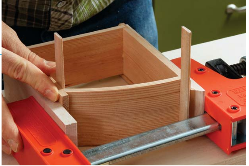
Attach braces and apply clamping pressure. A couple of pieces of thin stock backed with double-sided tape prevent the drawer front from pivoting as the clamp tightens.
