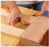
Wedge the supports against the drawer. Slightly longer than the distance between the supports, the wedge forces them against the inside of the drawer.
