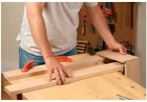
**Clamp supports to the top.** Align one support with the end of the bench. Place the second on the bench and slide the drawer over both. Push the second support against the back of the drawer and clamp one end to the bench.
