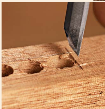
Chisel the mortise ends. Slip the tip of the chisel into the knife-cut line at the end of the mortise (above), then hold the chisel vertically and tap it with a mallet to begin squaring the ends of the mortise (right).
