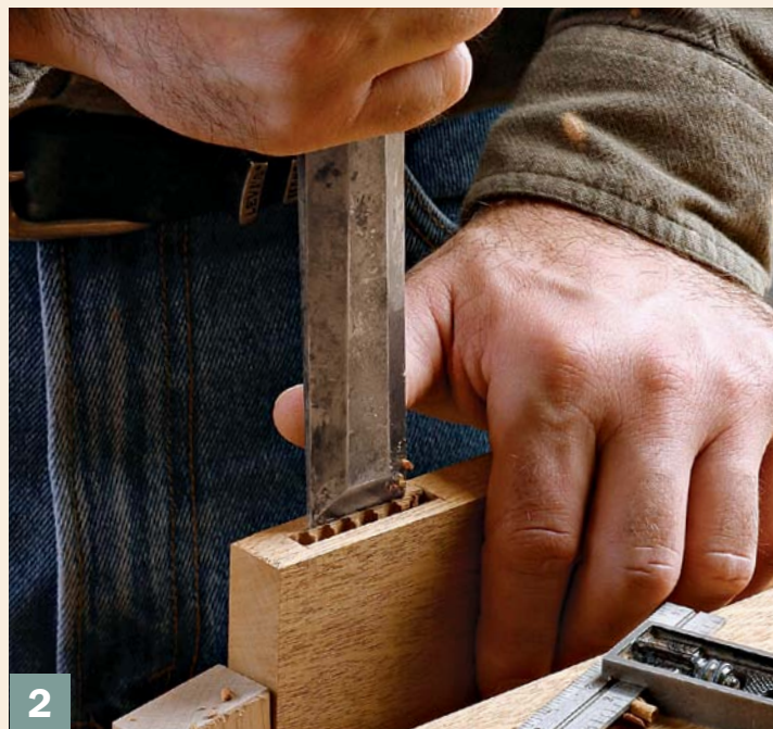
Clean up the sides. Chop out most the waste using a mallet, working from the middle toward the side. Then, using the knife line to register the tip of the chisel, pare the mortise sides flat and straight.
