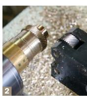
**Knurling.** After defining the neck of the knob, he creates a raised section and patterns it with a knurling tool, which doesn't cut, but operates solely by pressure.
