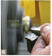
**Doming the infill.** With the knob mounted in his wood lathe, he turns the ebony infill to a smooth, slightly domed surface.
