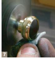
**This knob's finished.** After using sandpaper and Scotch Brite on the brass and wood, he applies wax and polishes the finished knob.
