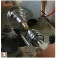
**Shaping and drilling.** With the raw brass rod held in a collet on his metal lathe, Rios Wong turns it to a clean cylinder, squares off the end, then drills and taps it.
