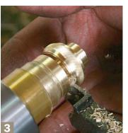
**Parting shot.** After turning bevels on either side of the knurled section, he parts the piece off the metal lathe.
