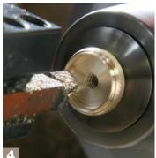
**Recess time.** With the knob reversed and held by its neck in a smaller collet, he turns a recess for the infill.
