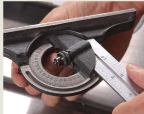
**Better than some other tools.** For angles other than  $90^\circ$ , a digital gauge will get you at least as close to  $45^\circ$  as a drafting triangle (left), and closer than the protractor attachment for a combo square (right).
