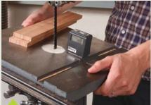
Sometimes it's the table that tilts. In this case, when angling a bandsaw table to cut dovetail pins, you zero the gauge on the blade (top), not the table. Stay clear of the teeth for a true reading. Then move it to the table (above) and dial in the angle.
