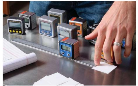
**Our best test.** With the gauge on top of a steel ruler, we then zeroed the ruler on a jointer table and began slipping strips of paper under one end. The best gauges allowed on average just four layers of paper before the reading changed from zero to 0.1°.
