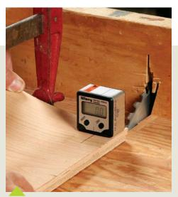
Works on workpieces, too. Michael Fortune uses his angle gauge to cut square edges on curved panels. He zeroes the gauge on the sled, and then puts the curved panel in place. Then he places the gauge halfway across his cutting line and tilts the panel to bring the gauge level.
