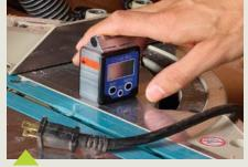
Dial in bevel angles on any blade. Zero the gauge on the saw's table (above), avoiding the throat plate. Then stick it on the blade in a plumb position (right) and adjust the tilt to any number you need.
