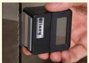
**Newest Wixey** has standout features. The tilt-up screen helps to defeat glare and saves you from bending over. A V-groove on the bottom registers the gauge accurately on a drill bit, and is surrounded by narrow magnets that fit nicely on the side of a typical bandsaw blade.
