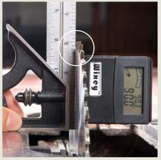
**Not quite as good as a good square.** You can tilt a tablesaw blade enough to see a tiny sliver of light in both directions without changing the numbers on the screen, demonstrating the margin of error inherent in these gauges.
