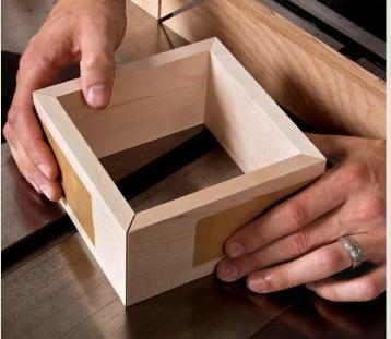
Often need test cuts anyway. No matter what setup tool you use, only test cuts will tell the whole truth. The trick is to get as close as you can beforehand, and a digital angle gauge does a very good job at that, with no bending over or squinting required.
