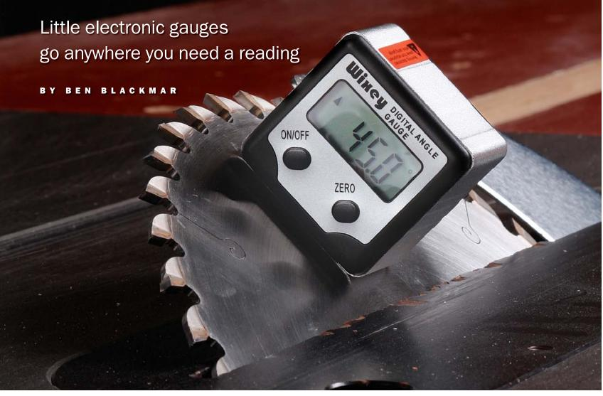
If you haven't seen them before, digital angle gauges, also called inclinometers, measure the angle of tilt after being zeroed to a reference surface. They have a magnetized base that attaches easily to most machine tables, fences, and blades in the shop.
