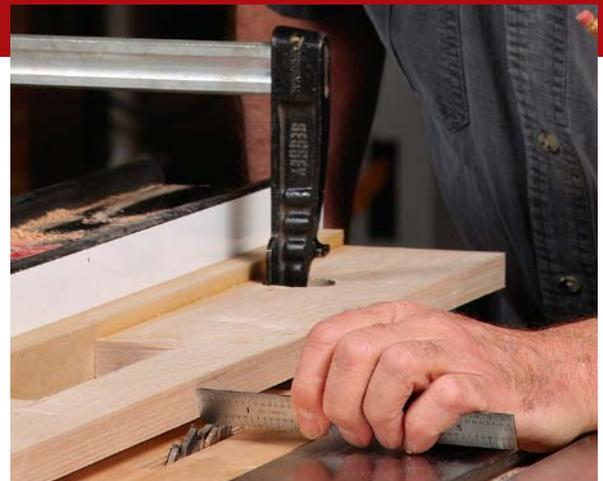
**Adjust the rip fence.** The width of the exposed dado set establishes the width of the rabbet. Measure from the edge of the L-fence to the outside of the blade's teeth.
