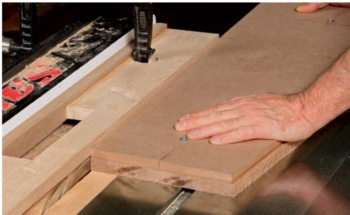
**Cut flush to the template.** Here, instead of using double-sided tape, the template is attached with screws, located in an area that will be cut away.
