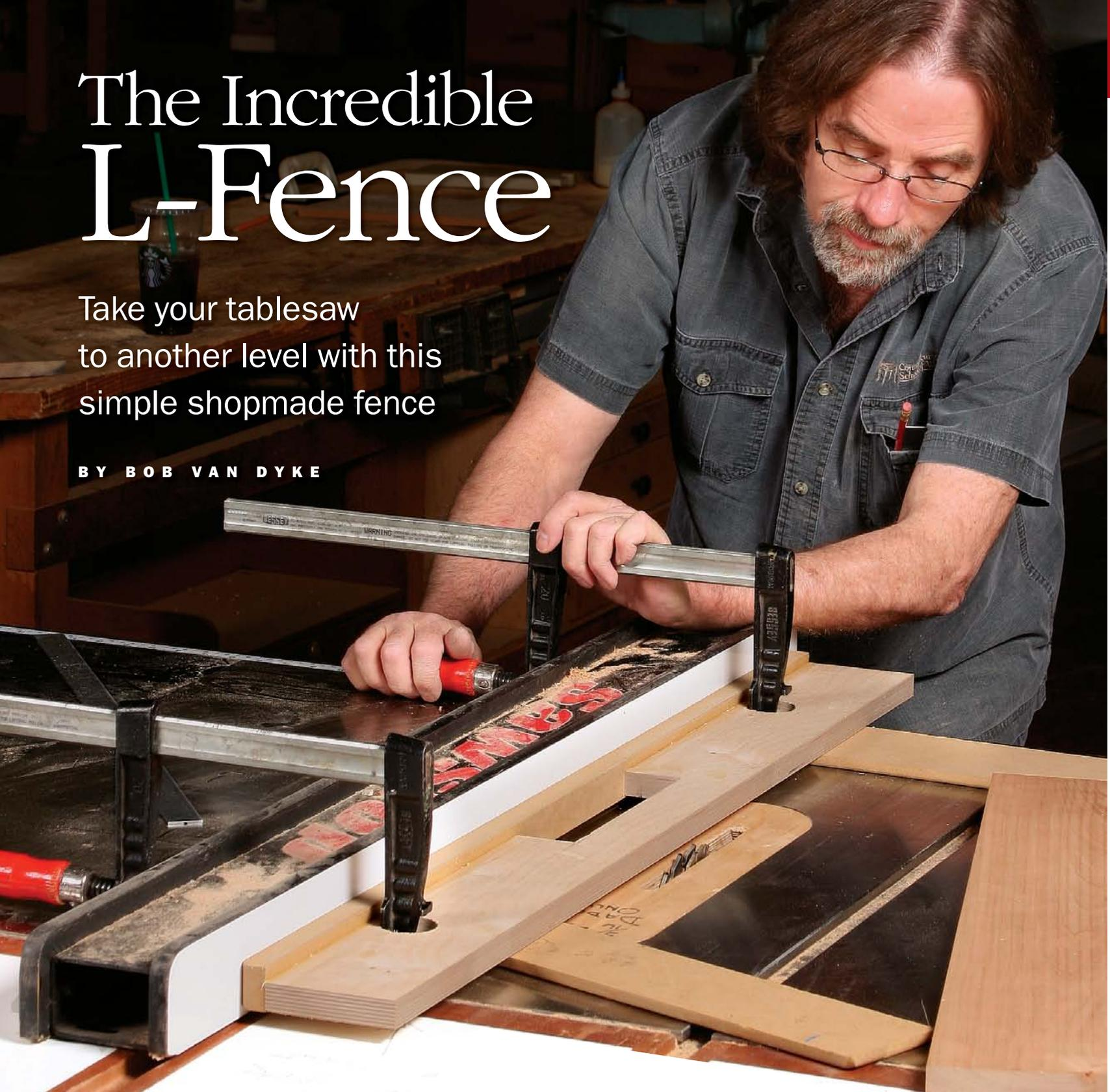
Adding jigs and auxiliary fences is a common way to increase your tablesaw's capabilities. But the most clever tablesaw add-on might be one you've never heard of. The "L-fence" makes rabbets, tenons, and straight flush-cuts a breeze, and it will change the way you think about miters. Once you grasp the basics, the L-fence will become an indispensable fixture in your shop.
