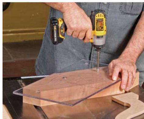
**Cut the critical edges.** After bandsawing away most of the waste, reattach the Lexan template (left) and use it with the L-fence to trim the critical edges (right). Afterward, use the leg pattern to mark the curves, and shape them any way you choose.
