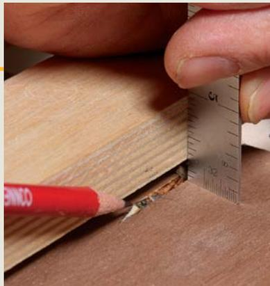
**Test cut sets up L-fence.** Tilt the blade to 45° toward the rip fence. Run a scrap from the case side stock halfway into the blade and hold it as you shut off the saw. Move the L-fence over the blade so its bearing edge is aligned with the kerf as shown.
