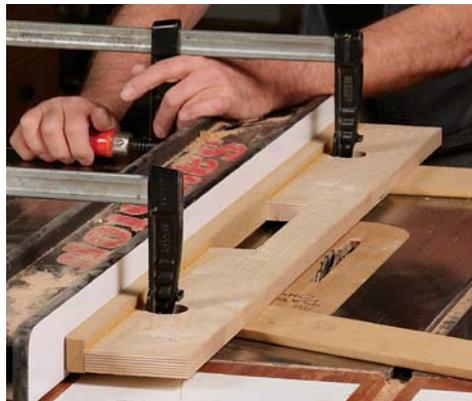
**Set it straight.** Set the L-fence  $\frac{1}{16}$  in. to  $\frac{1}{8}$  in. above the blades. Shims hold the fence parallel to the table while you tighten the clamps.
