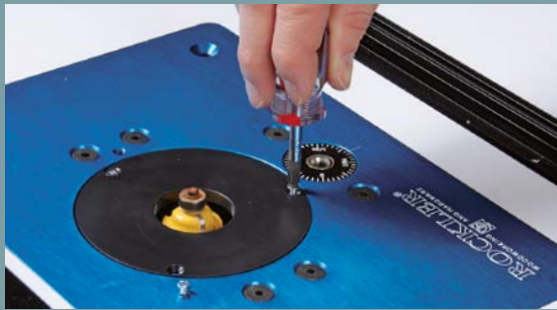
Twist and lock works well. Most of the lift plates use a spanner wrench to lock and unlock the insert ring. It's a fast and easy system.
