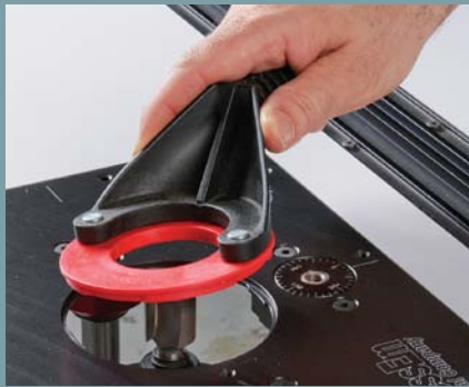
Twist and lock works well. Most of the lift plates use a spanner wrench to lock and unlock the insert ring. It's a fast and easy system.
