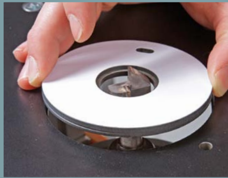
Snap-in rings are even easier. The insert rings for the Woodhaven EZ Lift have a rubber O-ring around them that keeps them in place. A screwdriver removes the ring.
