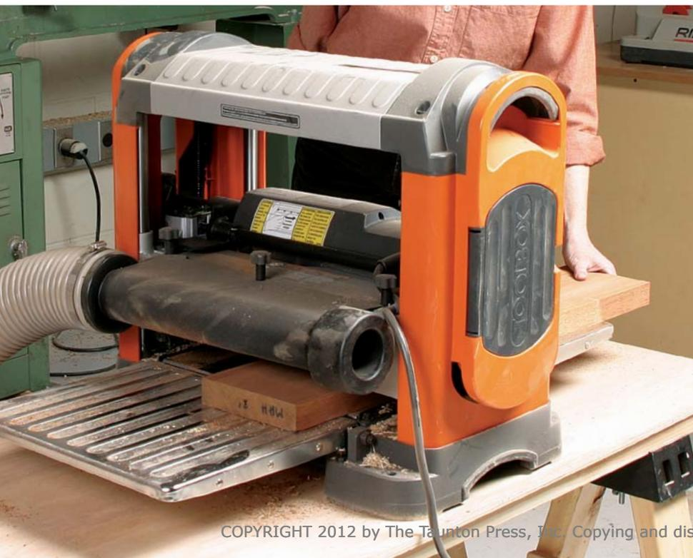
the board exits the infeed table because, for an instant, the guard doesn't cover the spinning knives.
