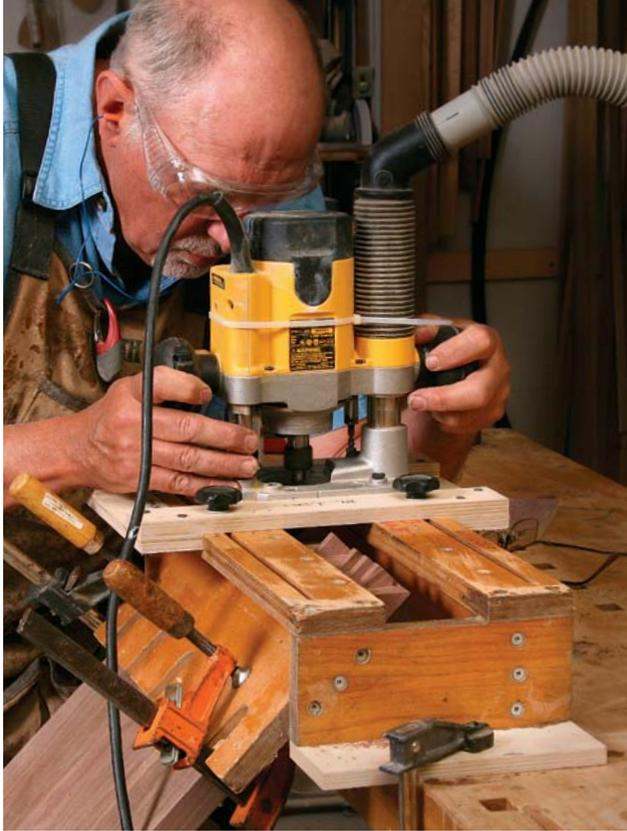
**Hog out the waste.** Lock down the carriage for each pass, staying clear of the knife lines. Cut to full depth with a series of light passes. Then creep up on the lines.
