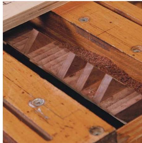
**Straight bit leaves the cheeks square.** The router establishes the mitered face of the joint but leaves the pin cheeks vertical—as if they were finger joints. The rest is done by hand.
