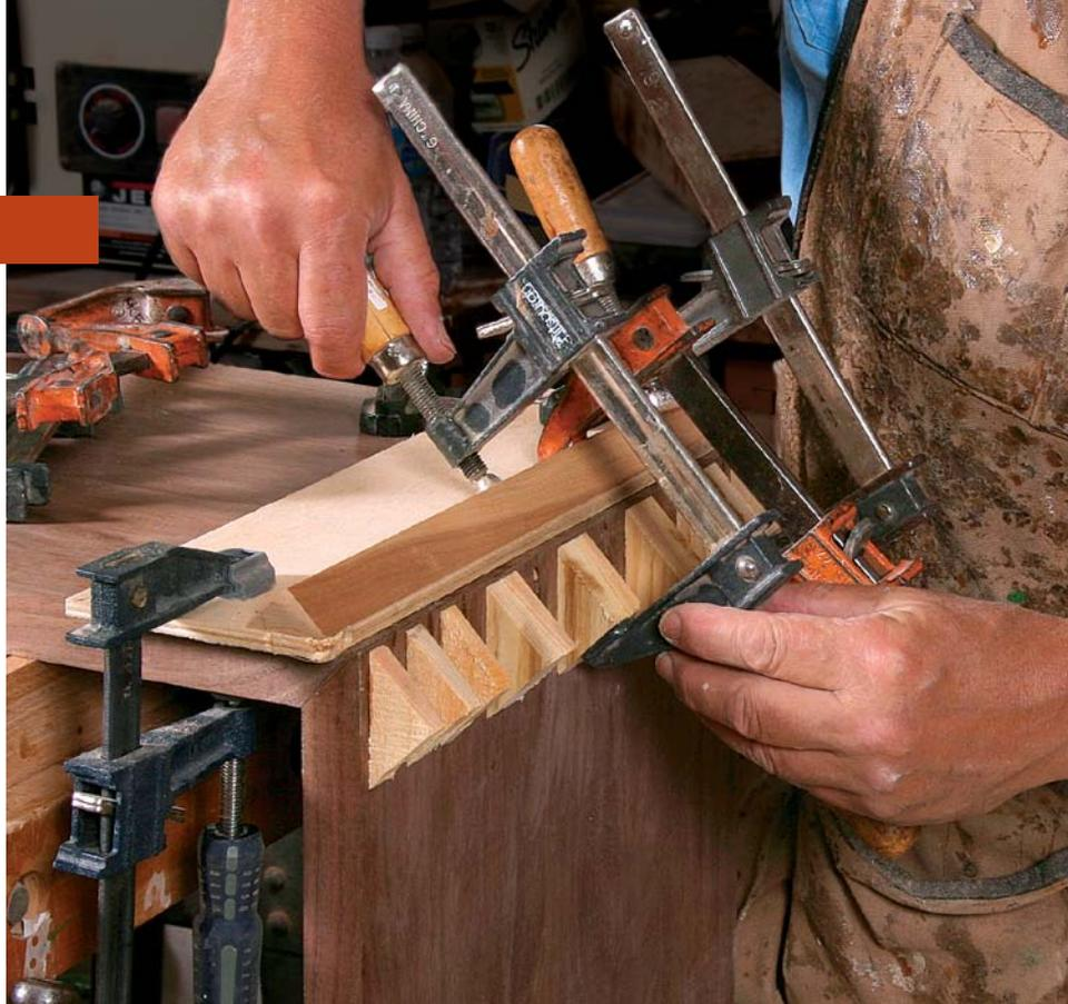
angle, and you simply rout with a straight bit between your layout lines. To avoid the look of template-cut dovetails, I cluster the pins at either side of the joint and use wider spacing in the middle.
