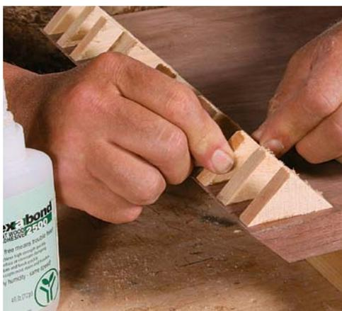
**How to clamp a half-blind miter.** Triangular clamping blocks adhered with quick-setting cyanoacrylate glue provide the purchase for clamps on the tail board. On the pin board, where the joint is blind, a long triangular block glued to a scrap of plywood (with sandpaper adhered below) and clamped in place does the trick.
