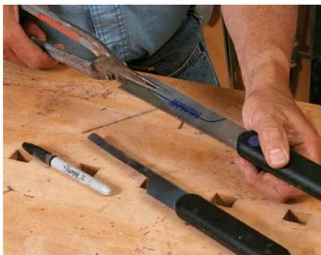
**New dovetail tool: tin snips.** To cut the angled shoulders of the pins, Fortune modifies a \$17 flush-cutting trim saw so it can fit between closely set pairs of pins.
