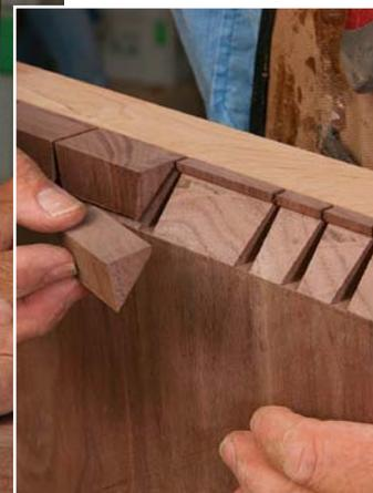
**Snap off the waste.** After the first cut, remove the waste pieces, then raise the blade for the final pass.
