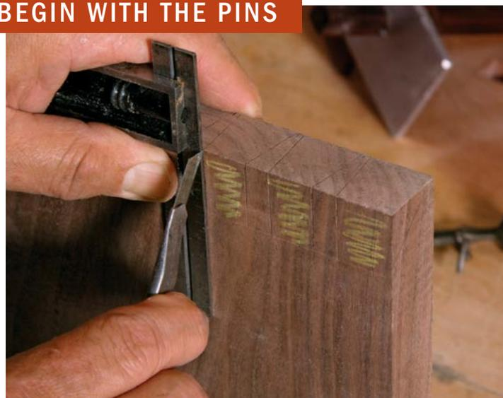
**Mark the pins with a knife.** Deep layout lines are essential to guide the routing. Don't lay out the miter so it comes to a complete point—leave a  $\frac{1}{32}$  in.-wide flat at the tip to allow for planing and sanding after assembly.
