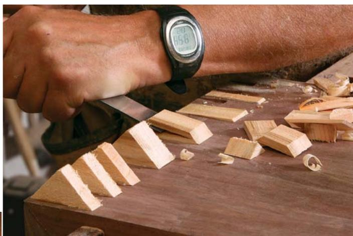
**Clear the decks.** After assembly, knock off most of each clamping block with a few quick strokes of a chisel. Finish the job with a handplane, being very careful of the mitered edge. Use sandpaper to produce the finished surface.
