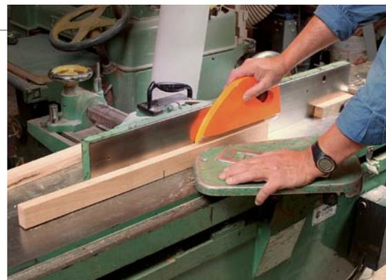
**Drop and go.** Put the caul against the stop block with a push stick hooked on that end, and lower the caul onto the cutterhead. Then push it forward. Do the same to the other end to create a gentle camber.
