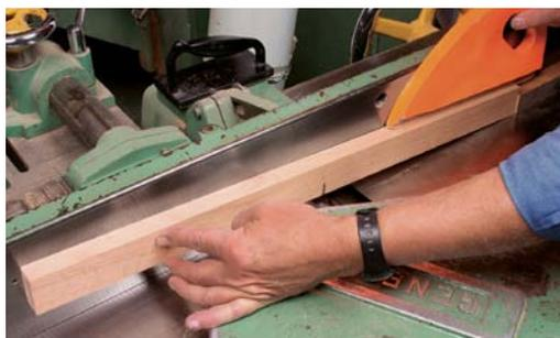
**Simple setup.** Mark the midpoint of the caul, and set up a stop block on the jointer so that point will drop right at the leading edge of the outfeed table. Set the jointer for a  $\frac{1}{32}$ -in.-deep cut.
