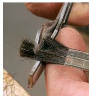
**Brush trick.** As is, cheap flux brushes are too floppy and tend to drop bristles into the glue. So hammer the ferrule to tighten up the bristles, and trim off some of the length.
