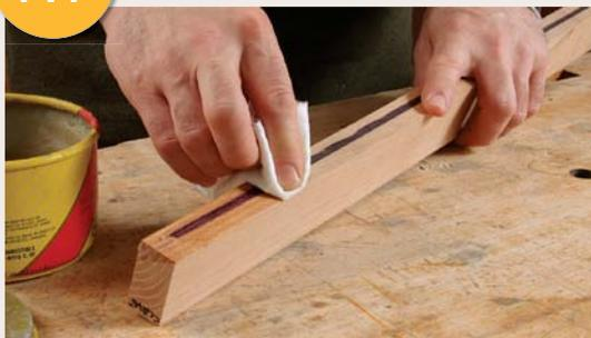
**Tape or wax.** The tape lasts indefinitely, but the paste wax needs to be refreshed from time to time.
