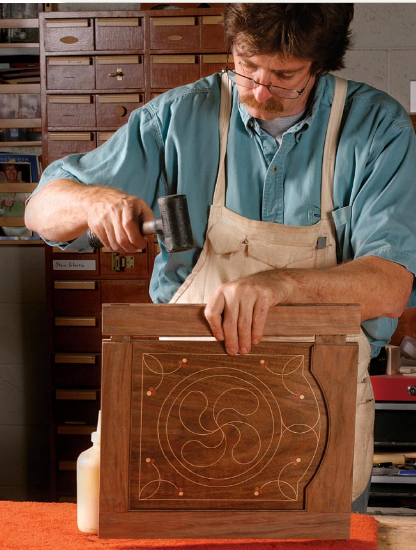
Sturdy frame for a picture-perfect panel. The door's inlaid panel slides into a frame joined with mortises and wedged through-tenons.
