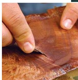
**Removing glue pockets.** Slice open the pocket (above), and then apply heat to the area with an iron (right). The heat will soften the glue, allowing the excess to seep out while the iron presses down the raised veneer.
