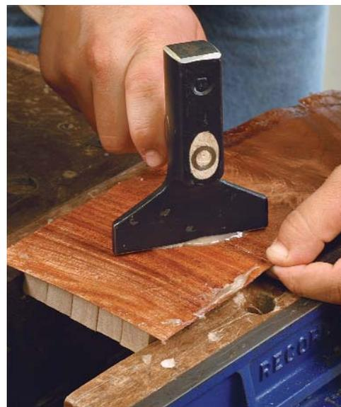
**Fixing air pockets.** Again, slice open the pocket (left), if necessary, work glue into the cavity (center), and then hammer down the problem area (right) for an invisible repair.
