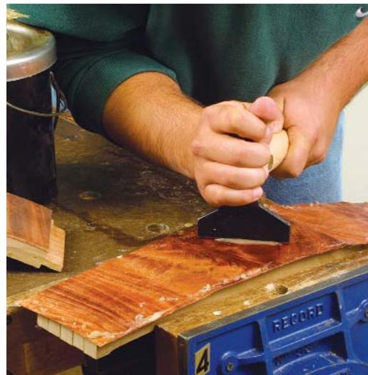
**Veneering goes quickly.** Position the veneer and apply glue to the top side to lubricate the hammer. Start from the center and work toward the edges, pushing out air bubbles and excess glue. Work the surface continuously until the glue cools.
