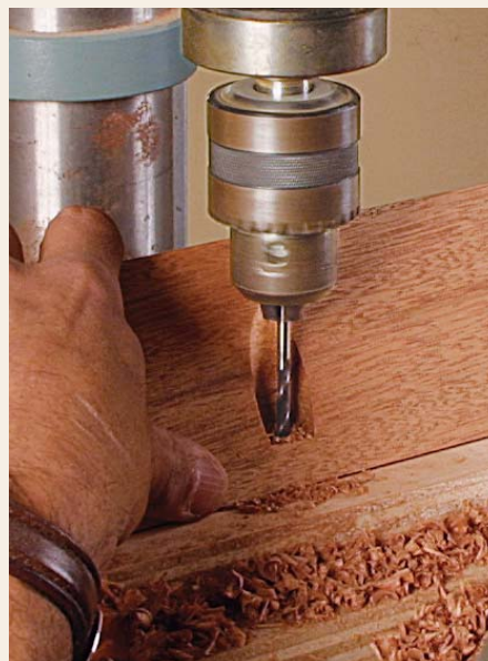
Pocket-hole jig. Construct a small jig to hold the rail at approximately 10° while drilling pocket holes with a Forstner bit.
