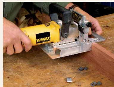
Grooves or slots. The clips are installed in grooves cut on the tablesaw or in slots cut with a biscuit joiner.
