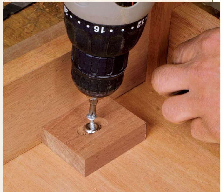
Room at the corner. Near the corner of the end rail, the block needs to have a slotted hole parallel to the rail. Make sure that the long grain, not the end grain, of the block is glued to the rail.
