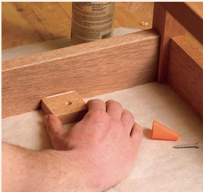
Attaching the block. With the rail sitting on a flat surface covered with wax paper, rub the glued block on the rail until it adheres. When the glue has dried, remove any paper that has stuck to the wood.
