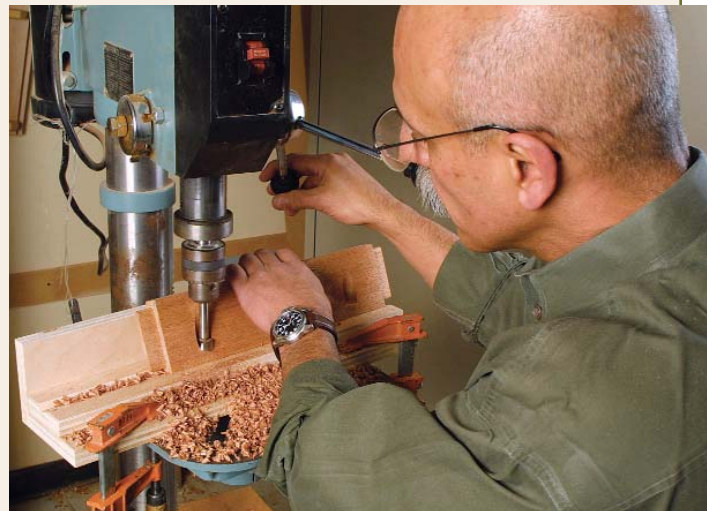
Pocket-hole jig. Construct a small jig to hold the rail at approximately 10° while drilling pocket holes with a Forstner bit.
