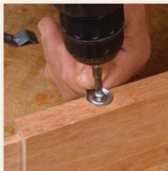
Attached to the rail. The twin-circle clips can be screwed to the rail either before or after the base has been assembled. Check that the clips are free to move.
