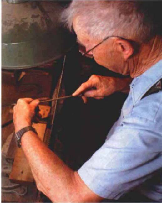
Aim for only half a shine at first. On the first pass (left), file the back of each tooth from the gullet up to the point, reducing the jointed flat by half. On the return pass (above), file the flats to sharp points. Remember that the only angle you change is the direction of the file.
