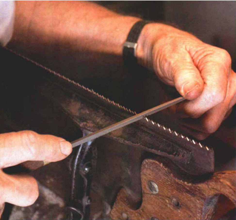
Aim for only half a shine at first. On the first pass (left), file the back of each tooth from the gullet up to the point, reducing the jointed flat by half. On the return pass (above), file the flats to sharp points. Remember that the only angle you change is the direction of the file.
