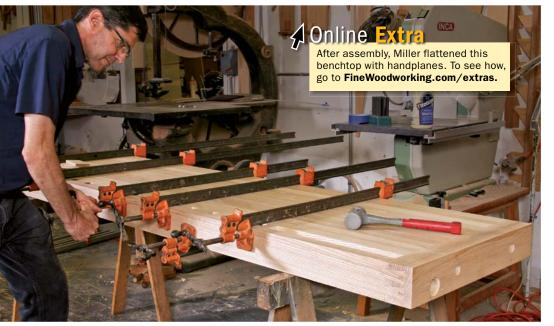
**Glued and bolted.** At final assembly, Miller bolted the end cap back onto the benchtop with no glue on the tenon. He glued the face board to the front of the top and to the end cap at the dovetail.
