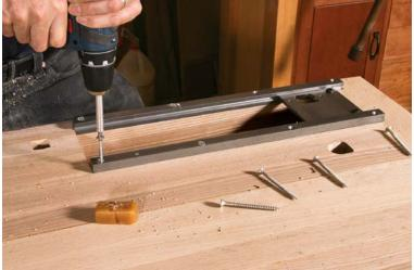
Two rails in one plane. To ensure that the wagon vise operates smoothly, its rails must be perfectly parallel and lie in the same plane.
