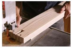
**Tails first.** Miller used the bandsaw (with a support stand to keep the long workpiece level) to cut the tails in the face board. The rabbet visible below the tails (above) provided better registration (right) when Miller marked the pins on the end cap from the tails.
