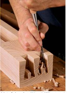
A lot of chopping. Although Miller started excavating the pins with a trim router, most of the wood had to be removed by hand.
