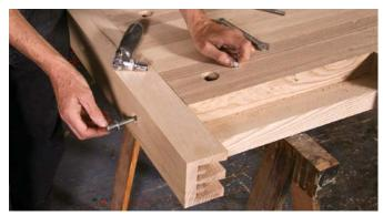
**Dry-fit the end cap.** The end cap is fitted to the tenon and bolted in place through oval clearance holes (above) to allow for seasonal movement of the top. With the cap in place, Miller used the Bench-Crafted template to mark it for the wagon vise handle hardware (right); then he removed the end cap and took it to the drill press.
