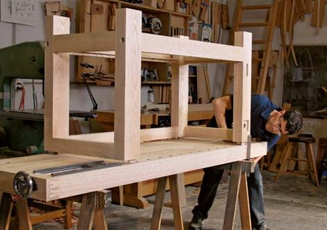
**Base and top must be flush.** For the leg vise to work properly, the front leg must be flush with the front of the benchtop. With the base aligned, Miller marked the position of the slip tenons in the leg tops so he could rout mating mortises in the benchtop.
