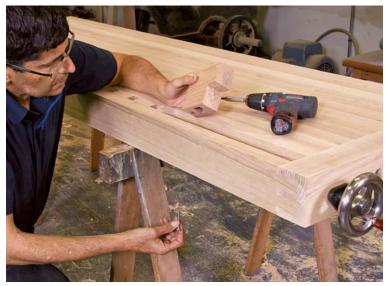
Drop in the dog block. With the benchtop flipped right side up, Miller fitted the dog block into its slot and fastened it to the moving plate with a screw from below. The nut block reinforces it well in use.
