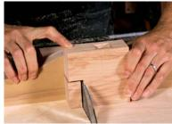
Save the extra dog hole. When the glue was dry, Miller cut the dog board to length. He used the extra dog hole (above) to make the moveable dog block for the wagon vise. Then he glued the dog board to the benchtop and planed it flush.
