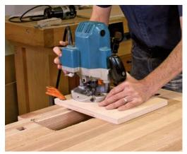
**Bridge the gap.** A wide sub-base screwed to the router provided the support so Miller could rout accurate grooves for the two wagon vise rails, working with the benchtop upside down.
