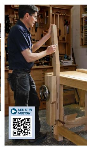
providing a solid grip unmatched by other vises. However, to do so, the leg vise incorporates an adjustable "parallel guide" at the bottom that must be set to roughly the thickness of the workpiece with a removable pin. The extra step takes a little getting used to, but the results are well worth it. BenchCrafted will soon have a new version of the leg vise available, at a higher price, with a scissor mechanism that will eliminate this step.
