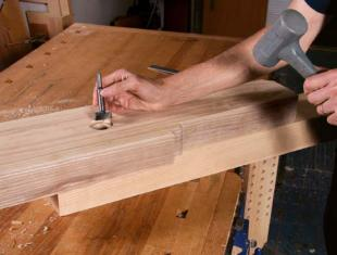
Drill before assembling the base. After using a Forstner bit to drill a hole through the leg-vise jaw for the vise screw, Miller used the same bit as a transfer punch to mark the front leg for drilling.
