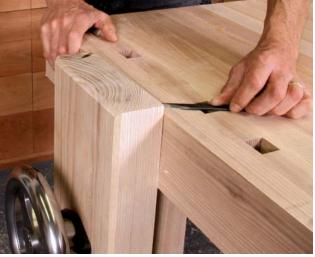
Correcting overbite. With the top flattened and the bench fully assembled, Miller marked the vise jaw so he could remove it and cut it flush with the benchtop.
