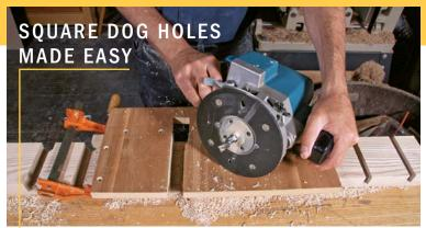
Dado and rout. After plowing out most of the waste with a dado set, Miller used a jig and router with a rub collar to create the benchdog slots. Then he added a facing board to close off the holes.
